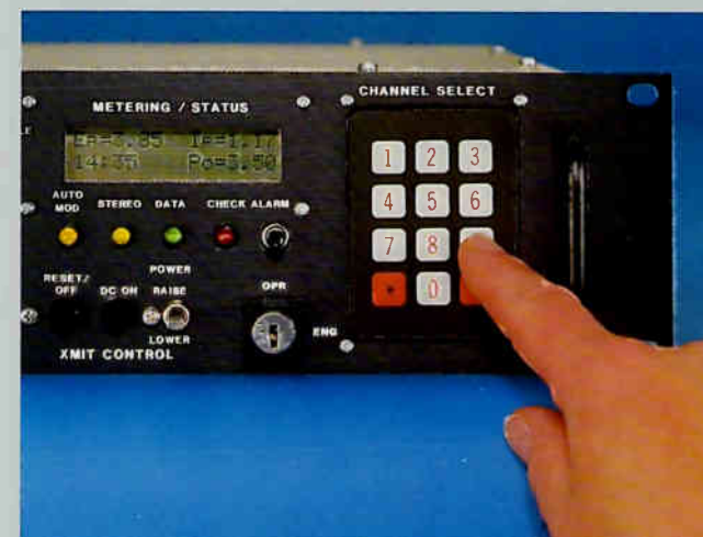
ARC-27 Studio Unit Controls and Display
