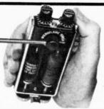
A completely self-contained gas welding torch that fits in the palm of your hand and produces 5000° F. pin-point accurate flame. Welds, brazes, solders—hundreds of uses in the shop, jewelry repair, dental labs, tool and model making . . ideal for silver soldering and printed circuit repair—anywhere precision high heat is required. Easy to operate. Complete with torch, 3 tip sizes, 1 each compressed butane and oxygen cartridge. Shpg. wt. 1 lb. \$17.95
