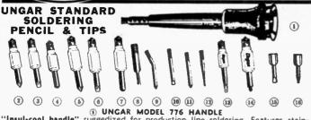
\*\*Insul-cool handle\*\* ruggedized for production line soldering, Features stainless steel deflector for low handle temperature, ceramic and glass insulation for longer life, tough phenolic for added durability and extra heavy, extra flexible 6 ft. 18 gauge polyvinyl cord. Cork finger-grip, red colored handle. Accommodates all elements and tips below.
