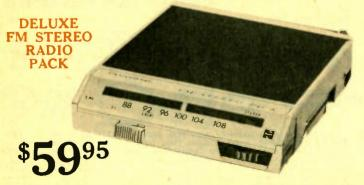
Plugs into any Panasonic car stereo player for full range FM stereo multiplex over your regular speakers. Tunes 88-108 MHz. Operates on 12 V. negative ground, supplied through tape player. Highest quality Panasonic design employing 15 transistors and 11 dlodes. Wt. 1 lb.
