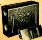
Compact single unit with exciter lamp, photo-cell tube, and two lenses. Projects a beam of light across any entrance from 3 to 20 ft. in daylight. Mirror reflects beam back into photocell. Breaking of this beam by any person or moving object operates built-in relay which in turn sounds chime furnished. Perfect for professional offices, stores, factories, homes—anywhere. Grey hammertone metal case, size only 8%x61/2x23%". For 115 volts, 60 cy. AC. Shpg. wt. 8 lbs.
