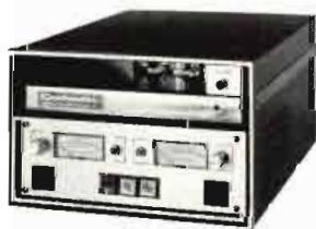
1070RPS – Stereo record/playback with Phase-Lok II head bracket to eliminate FM phasing problems. 1070SDL – Stereo delay programmer.
