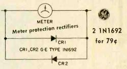
The New General Electric \$1.50 Manual no. ETR 3960 show how the above meter protection circuit works. 200 pages
