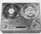
Model 64X. Plays/records 4-track stereo or mono through home system. Separate record, play, erase, bias heads. Bias head gives hi-fi response even at slower speeds. Tape monitoring and sound on sound. Level "eyes" and automatic shutoff. 7½, 3¾, 1½ ips. 20-25,000 Hz at 7½ ips. Flutter/wow. 0.15%. Teak case, 15¾x11½x65%. AC. Imported. 15 S 7650 Z. Shpg. wt., 23 lbs.....
