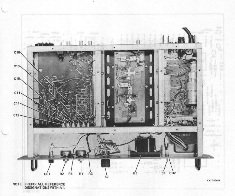
Figure 5-2. FM-15QE Exciter Bottom View with Cover Removed.
