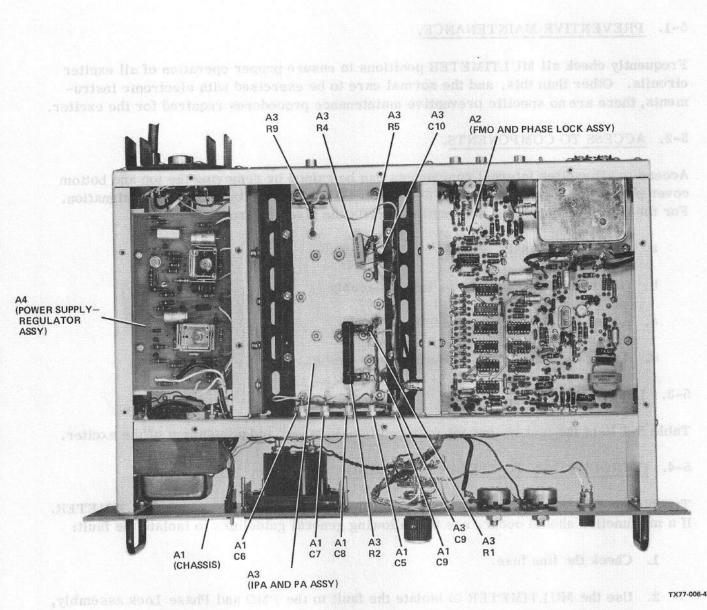
the IPA and P's assembly, the Power Supply-Regulator assembly, or to chassia
