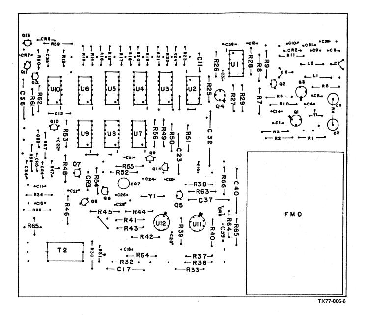
Figure 5-3. FMO and Phase Lock Assembly, Location of Parts.
