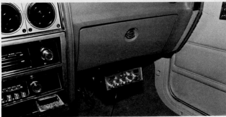
The final mounting position used here was the passenger's side of the front seat.
