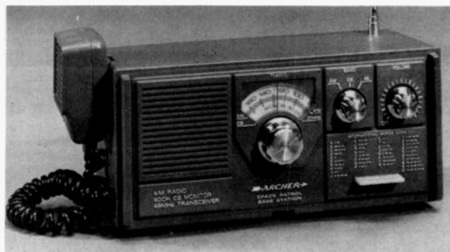
Some interest has been noted in Part 15 hobby potentials by a few manufacturers. This current Part 15 AM/CB "base" station operates on 49.86 MHz. It is an Archer product sold through Radio Shack stores.
