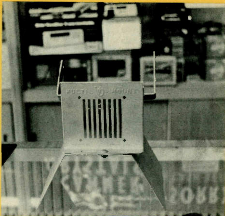
A universal mount is available for your rig. Like a hump mount, it sits astride the transmission tunnel, but it usually doesn't include an integral speaker. (Marc Stern photo)
