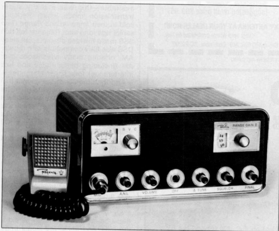
Double Sideband (reduced carrier), also known as DSB, was used in this Regency Range Gain II CB rig. While totally compatible with AM stations, it offered many of the advantages of SSB and avoided many of the problems and inadequacies of AM. Today CB'ers have a choice of AM or SSB. They ask about DSB—but nobody makes these sets anymore!
