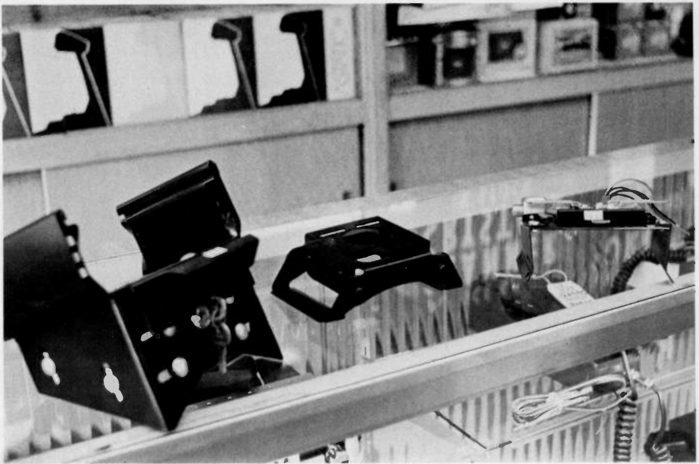
A variety of mounts are available to protect your rig. You can use one of the hump slide mounts shown or one (left) with a lock for greater protection. (Marc Stern photo)
