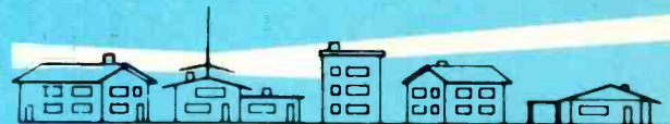
Ordinary collinear or ground plane antenna signals are blocked...they radiate from the bottom.
