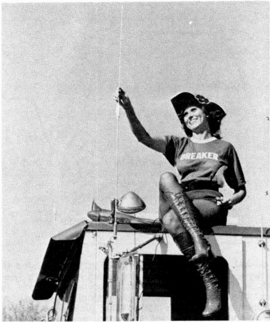
Fig. 4—The CB quarter-wavelength "whip" antenna (which is normally over 100 inches long) is compacted into a shorter length by the addition of a loading coil at antenna center. This compact whip is intended for truck use where the over-head clearance is marginal (Photo courtesy of Breaker Corp.).
