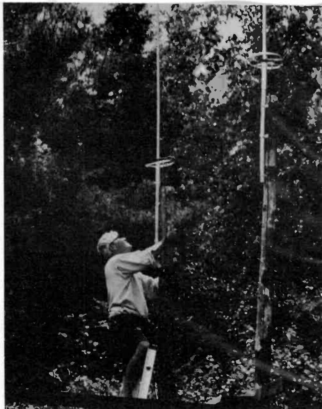
Co-author Atchley makes an adjustment to one of the four Ringo Antennas.
