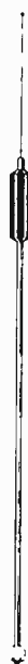
Fig. 3—The Masley CT-2 "Tarantula" whip is representative of the compact, center-loaded mobile antenna. The whip is only 54" high. The missing portion of the antenna is wound up into a coil placed at, or near, the mid-point of the antenna. Center-loaded antennas are to be preferred to base-loaded antennas, as they have greater efficiency. The tip section of the whip is adjustable, permitting the whip to be used over a wide range of frequencies.
