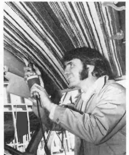
Make sure you know what you're drilling into. A high-speed drill can easily tear up other electrical wiring or even worse, bore through the van's roof!
