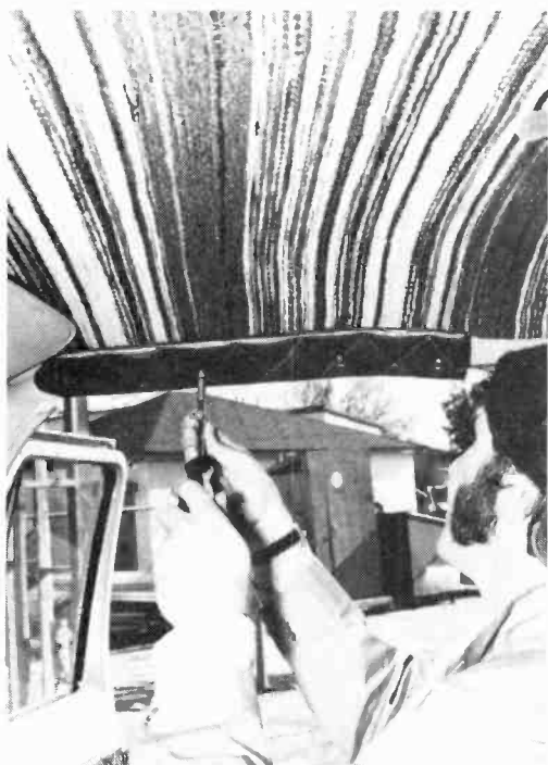
Remove the screws that hold the headliner in place.
