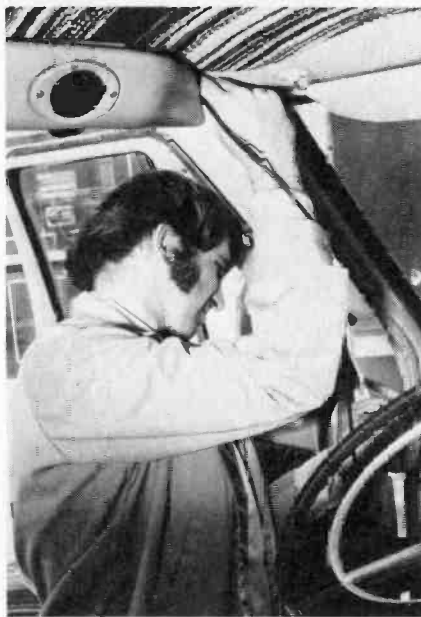
Once the coax is located, gently pull the slack through and again work it into an area hidden from view.
