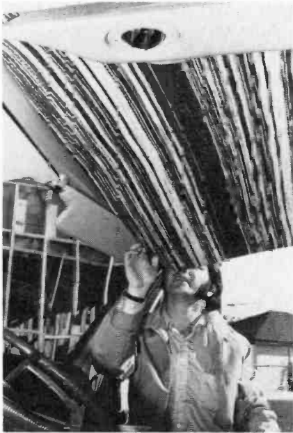
Pull the headliner down slightly to locate the coax cable. Sometimes a straightened coat hanger is useful in pulling the coax through.
