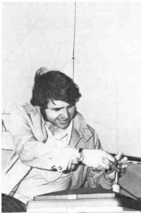
Connect the base-loaded coil and antenna to the mounting bracket. Using the Allen wrench that comes with antenna kits, securely fasten the antenna to the coil.
