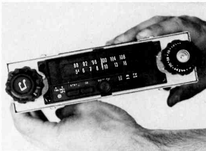
Before you go through the trouble of installing the unit in your car, hook up the wires and speakers to make sure everything works.
