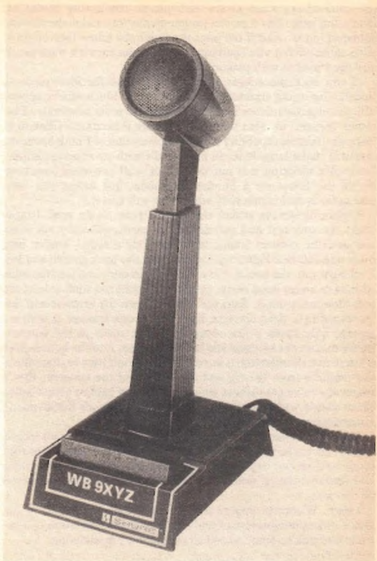
A desk mike for use with a home base. The PTT bar is across the front of the base.
