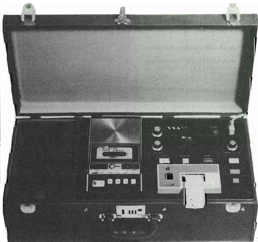
Bottom. An anti-bug system comprising tap detector, tap defater, telephone monitor and scrambler.
