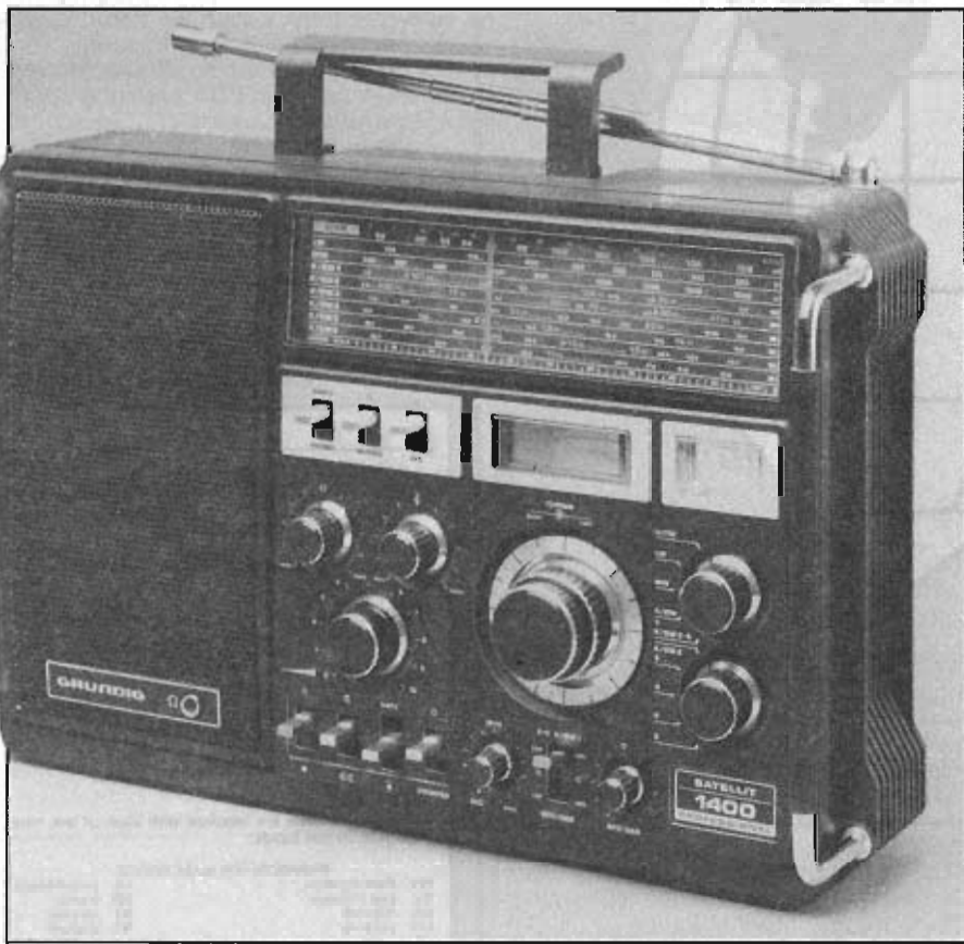
The Grundig Satellit 1400. Digital frequency readout and covers 1.6 to 28 MHz. Approx £250.
