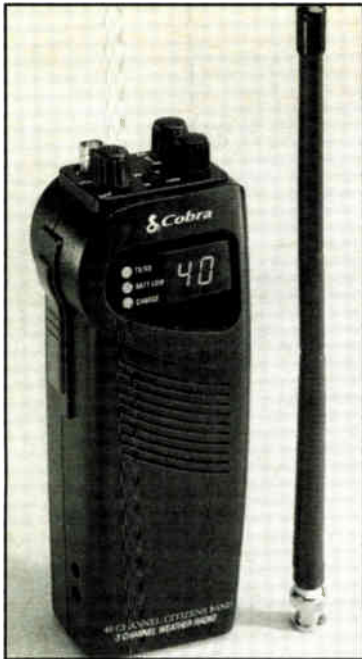
Your handheld CB, such as this Cobra HH 35-WX can be a lifesaver during severe weather. It receives NOAA weather broadcasts and features a BNC antenna connector. (Courtesy Cobra Electronics)
