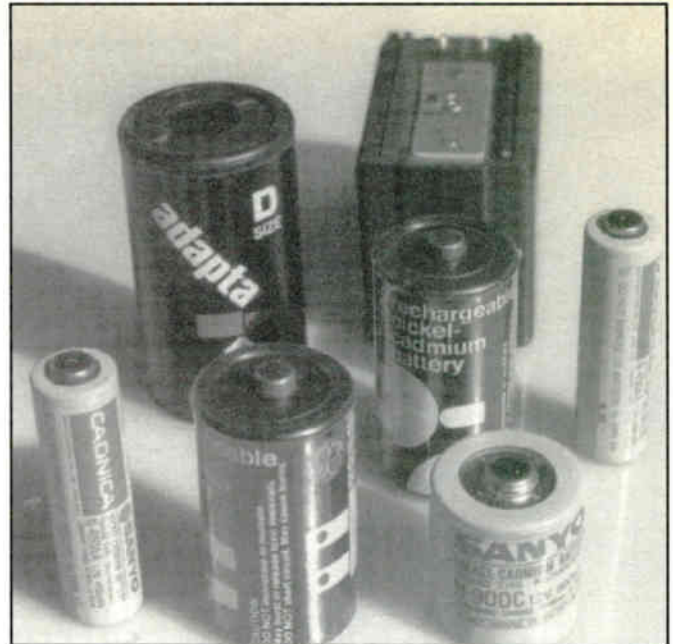
Here's a variety of rechargeable NiCd batteries; the smaller diameter "AA" cells are the most common ones used in CB electronic portable sets.
