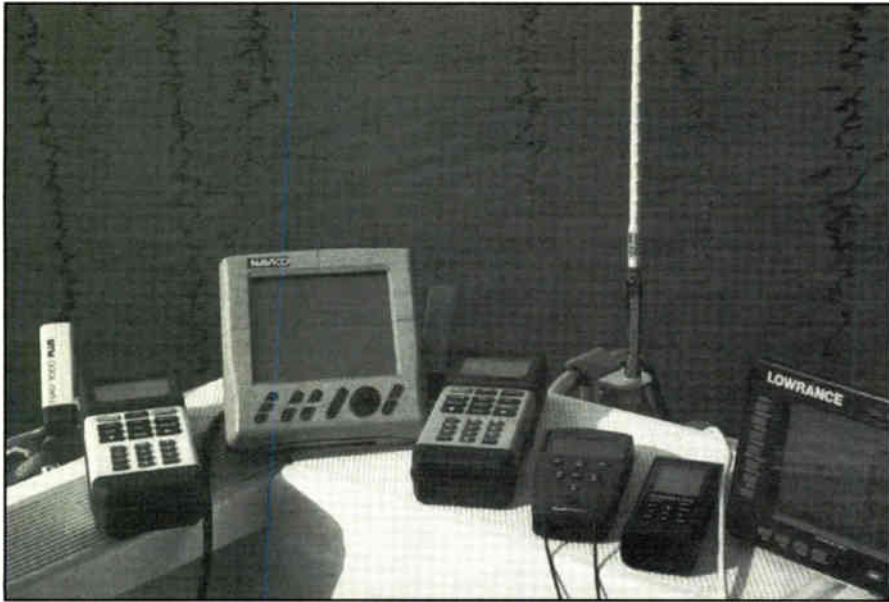
Portable GPS navigation receivers work off "AA" alkaline cells. Remember: alkalines are your best bet if you're going to be away from a power source used to recharge NiCds.
