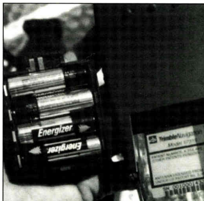
Double-check your springs to make sure they aren't getting rusty.
