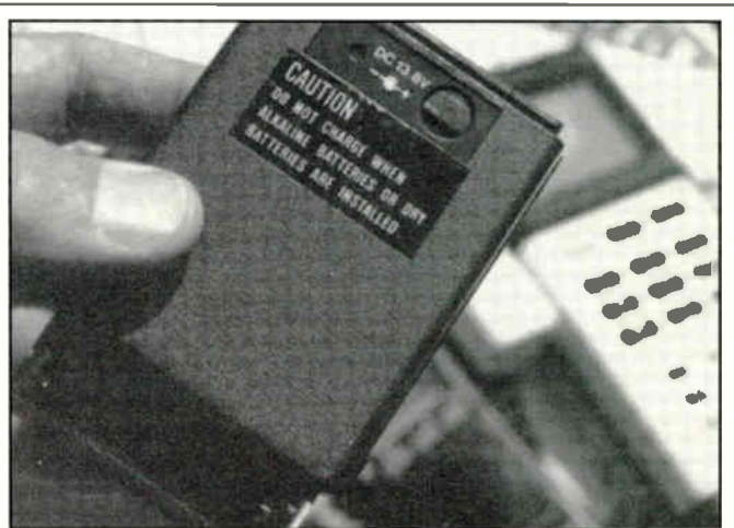
ALWAYS check the jack/plug polarity before you plug in an external 12 volt source.
