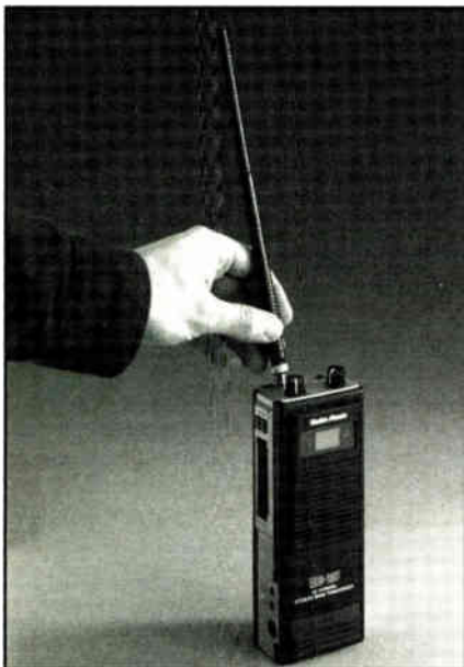
The ideal CB walkie talkie will have a BNC antenna connector on top. This way, you can easily remove the rubber duck and by using a simply SO-239/BNC adapter, use your mobile antenna.
