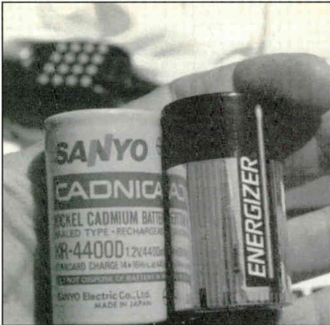
The rechargeable cell (left) will only give half the life as the alkaline cell on the right.
