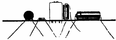
Figure 1 Component leads bent slightly outwards to hold them in place prior to soldering.
