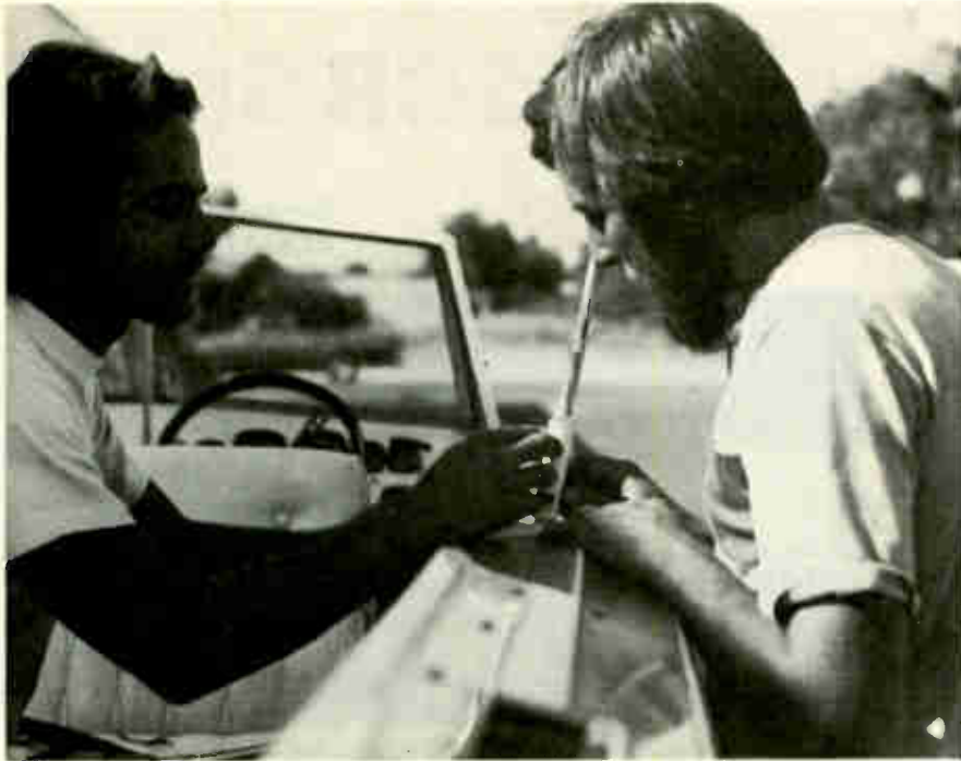
Technicians installing an antenna that requires no ground plane on the small craft.
