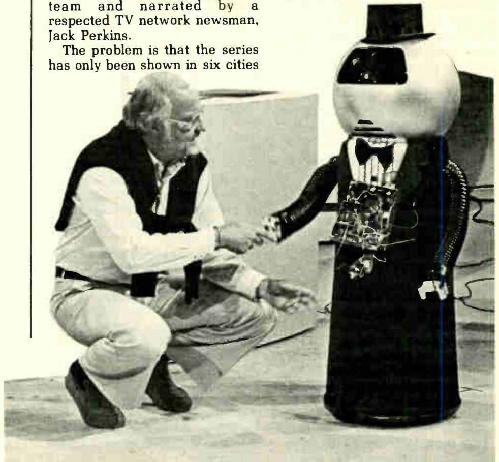
Jack Perkins, left, welcomes Orion, a UHF radio-controlled robot as co-host of a program for CB radio fans titled, "Give Me a Break." Orion walks, talks, shakes hands, tips his hat, and can key a CB mike.
