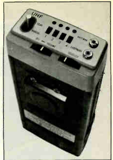
Designed for use in the field, away from mobile communications, the Realistic Pocket-Scan may be used to monitor any four of the available GMRS channels.
