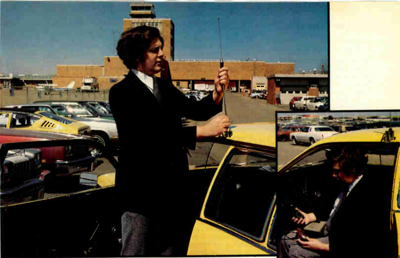
Above: A gutter-clamp antenna can be quickly fastened to a rental car and the coax fed in through a window. Be careful to avoid crushing the cable when the window is rolled up.
