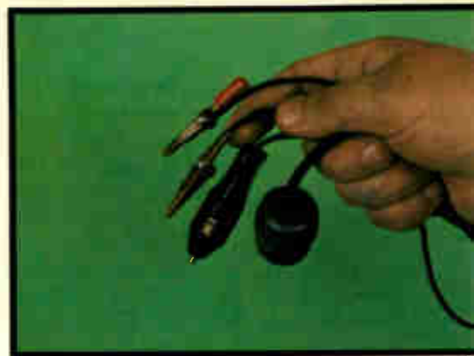
Adaptor cords are the key to getting power in strange cars. A cigar-lighter adapter, as well as a set of alligator clips insure the availability of DC power in any car.
