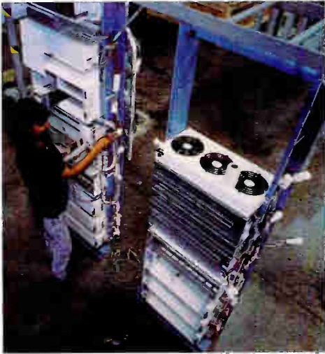
A customer-defined fiber optic termination bay is assembled.
