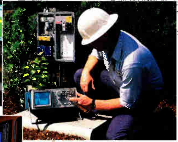
(ABOVE) THE 2714 CABLE TV SPECTRUM ANALYZER AUTOMATES ALL COMMON CABLE SYSTEM SPECTRAL MEASUREMENTS, INCLUDING THE FCC RF PROOF-OF-PERFORMANCE REQUIREMENTS.
