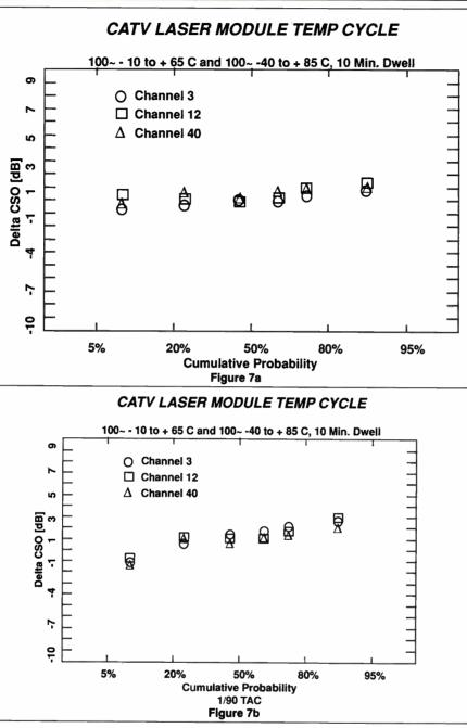
subjected to end of life aging (EOL) and to long term aging (LTA). Mean lifetimes of greater than 40 years are expected with respect to increases in second order distortion. In addition, no measurable change of RIN occurred for these populations.
