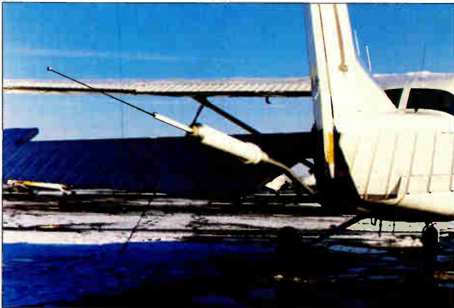
The rear of Flight Trac's Beechcraft Dutchess aircraft, showing the protruding antenna system.
