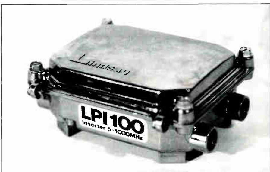
Lindsay, among others, has developed passives that will handle 1 GHz.
