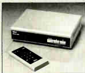
Oak's Micro 550, a 550 MHz, 83-channel remote control converter
