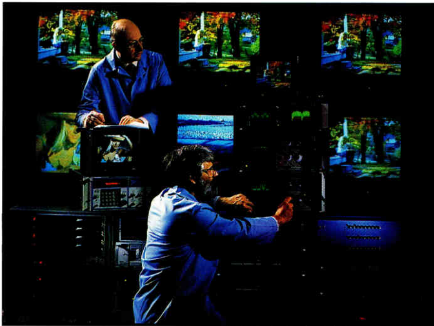
Engineers in Glenview, Ill., test the Zenith "Spectrum Compatible" HDTV transmission system. Today's cable and broadcast transmission systems can cause interference, as shown in the bottom row of TVs being tested by Zenith's Wayne Luplow, left, director of electronic systems research and development, and Rich Citta, manager of electronic systems research and development.
