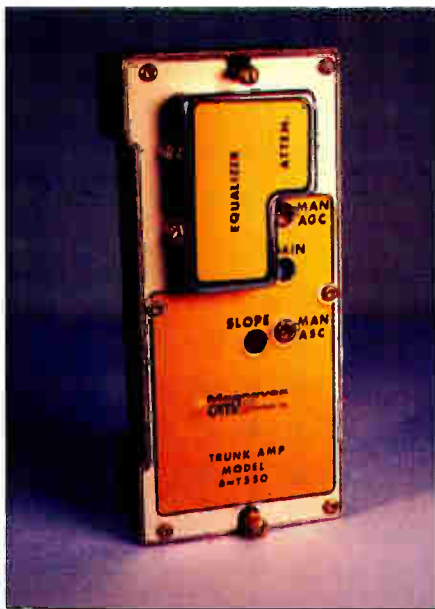
Magnavox's power doubling module
