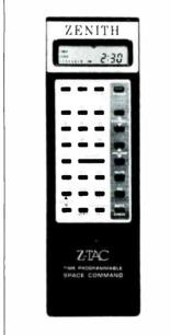
The TAC-Timer programs Zenith's Z-TAC decoder for multiple channel VCR recording.
