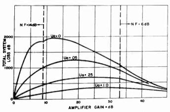
Figure 4. Achievable system loss versus amplifier gain for various "uncertainty" figures showing the effect of the assumed variation of noise figure with gain. Compare with Figure 2.
