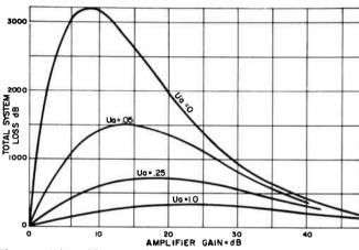
Figure 2. Achievable system loss versus amplifier gain for various "uncertainty" figures. The idealized amplifier has the same parameters as in Figure 1.
