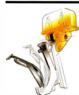
Our unique eight-point suspension and hinged drop chute with removable gate isolate vibration from the machine and cable. Service loops can be restrung without cutting or splicing. And only Case offers a front trencher, rear plow combination.
