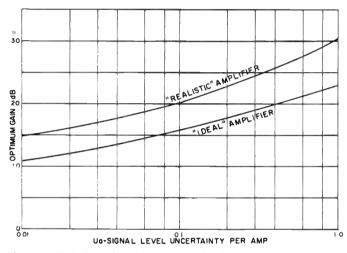
**Figure 5.** Variation of optimum gain with level uncertainty for the idealized amplitier and when the noise figure is a function of gain.
