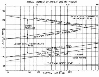
Figure 1. System level and tolerance diagram. Amplifier gain 8.69 dB. Output capability 50 dBmV. Noise figure 9.2 dB. Signal-to-noise ratio 40 dB.
