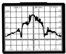
Reference Satellite Video Signal with Interference for C/I = 10 dB and with IF Filters at 60 MHz and 80 MHz
