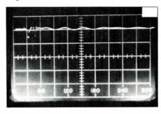
Figure 6. Return loss of 100 ft. RG-59 terminated in 75 ohms
