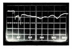
Figure 11. Return loss of a converter tuned to channel 4/100 ft. RG-59
