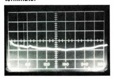
Figure 4. Return loss of an open
