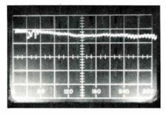
respectively. Figures 6, 7 and 8 show test results with a length of good drop cable. It is relatively easy to see what would happen to the various ripples and bumps with a length of cable which has some structural deficiencies. Figure 9 shows the test results of a length of bad cable terminated with the test resistor.
