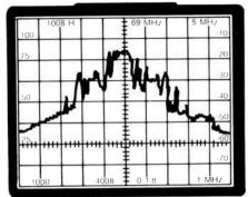
Reference Satellite Video Signal with Interference for C/I = 10 dB
