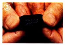
Check the braid impression on the underside of the removed jacket. A deep impression indicates a jacket which is too tight. This may cause difficult "F" connector installation. An extremely shallow impression indicates a jacket which is too loose.
