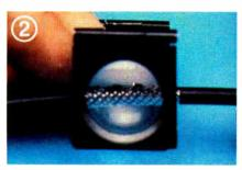
Carefully strip jacket off one inch of cable. If you ordered 67% braid, make sure 2/3 of the foil is covered by braid—not 1/2 or less.
