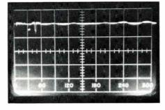
Figure 5. Return loss of a short
