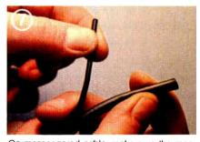
On messengered cable, make sure the messenger separates without tearing into the jacket and exposing the shield.
