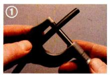
Measure the overall outside cable diameter with a micrometer. If it is not .242", connectors may not fit properly and performance might be affected.
