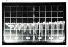
Figure 7. Return loss of 100 ft. RG-59 shorted
