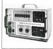
the nature and severity of the fault. It will detect opens, shorts, frays and crimped cable as well as faults in splitters and can also be used to detect faults and accurately find the length of cable while still on the reel. It will "look beyond" discontinuities on a cable, or beyond several splitters or other in-line devices, to find faults further along the cable run. Unauthorized connections to CATV drops can be detected even when isolated with a splitter.
