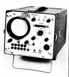
The Model 600, using the Time Domain Reflectometry Principle, has a range of 75 miles and accuracy of ±0.5% of range. A single sinusoidal pulse is generated at different repetition rates depending on the size of the loading coil. High sensitivity results from a variable output to 60 volts and gain to greater than X1000. The Model 600 is fully portable and operates either from line voltage or internal rechargeable batteries, giving up to 5 hours continuous operation.
