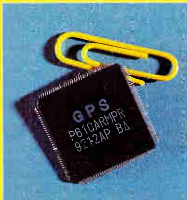
Photo A: The remarkable size of the ARM 610 is only apparent when compared directly with a universally recognizable object. GPS (GEC Plessey Semiconductors) recently became the second source for the ARM processor range.
