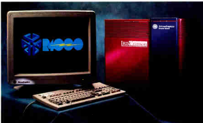
The Iris Crimson introduces the R4000 processor from Mips Computer Systems and Silicon Graphics' Elan graphics card.
