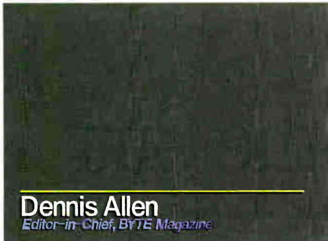
Photo 1: The first step in video titling is creating a graphics file with a background made up of the key color—in this case, black.
