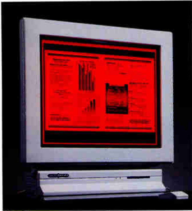
Photo 2: ACPDPs are produced in a wide range of sizes. They are bright, have good resolution, and come in thin packages. Small ACPDPs work well in instrumentation and portable computers. Large ACPDPs can display a lot of information at one time, which makes them good for use in computer terminals, CAD displays, and command-and-control applications. (Courtesy of Electro Plasma)
