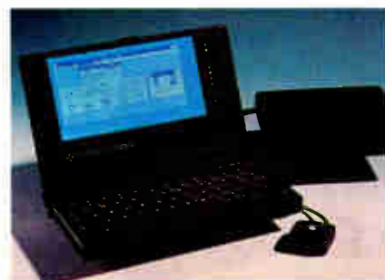
Photo 2: The Dell 320SLi is a robust 4-pound sub-notebook. Its performance and many of its components match those of heavier 386-based notebooks.
