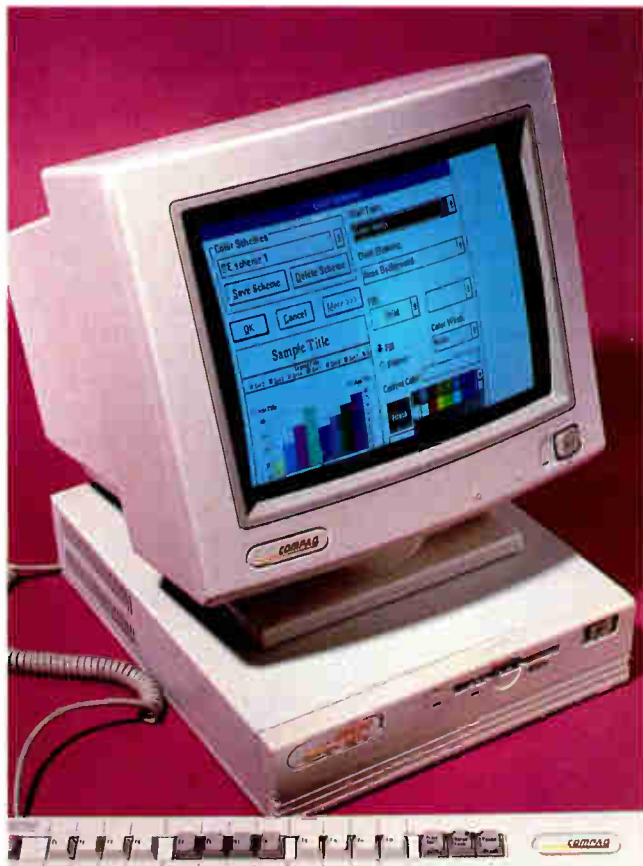
The Compaq ProLinea 3/25s is one of two 25-MHz 386SX models intended for users with limited budgets and experience.
