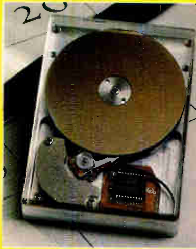
Photo A: Hewlett-Packard's new Kittyhawk 1.3-inch hard drive will give manufacturers of hand-held computing devices more flexibility in design. Available in capacities of up to 21.4 MB, the Kittyhawk is less expensive and uses less power than solid-state memory cards.
