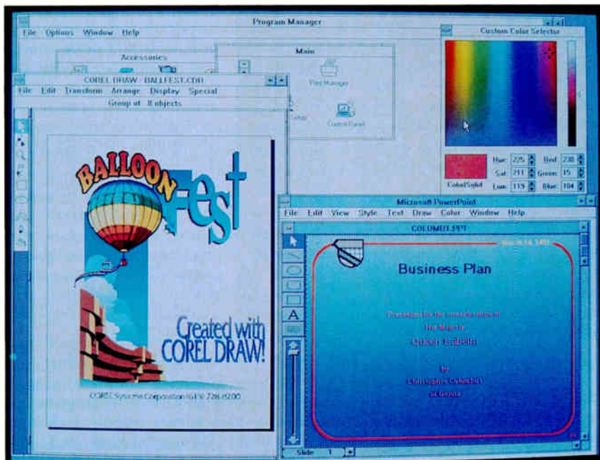
Photo 2: A 24-bit display. With a 24-bit graphics board such as the RasterOps 1024MC, Windows 3.0 doesn't have to resort to dithering or approximations; it outputs the true colors called for by the application.
