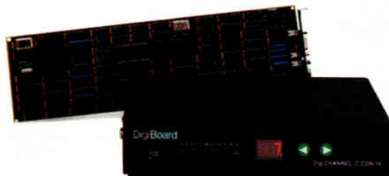
DigiCHANNEL C/X System. Connects up to 64 users to the Host Adapter Card via up to 4 intelligent DigiCHANNEL C/CON-16 concentrator boxes. Provides 38.4KB performance for all 64 users.
