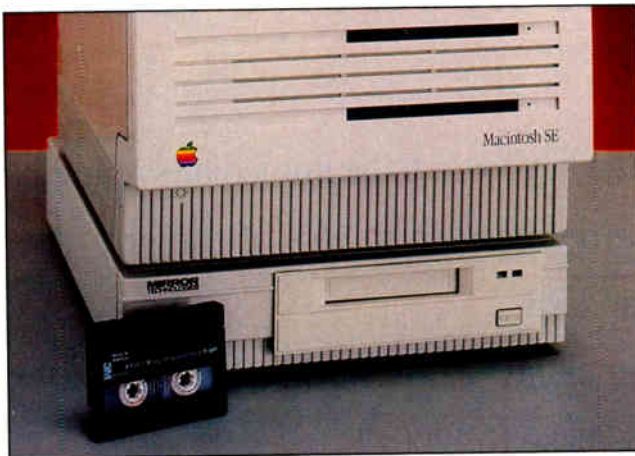
Mirror's T1200 DAT drive offers Mac users unattended backups, 1.3 gigabytes of storage, and high-speed access to data.
