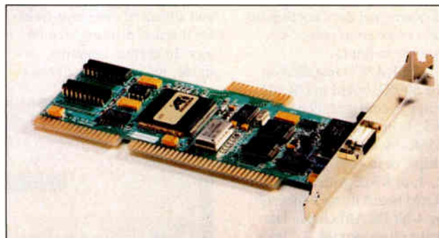
The VGABASIC-16 delivers 16 bits on a card that measures 6¼ by 2¾ inches.
