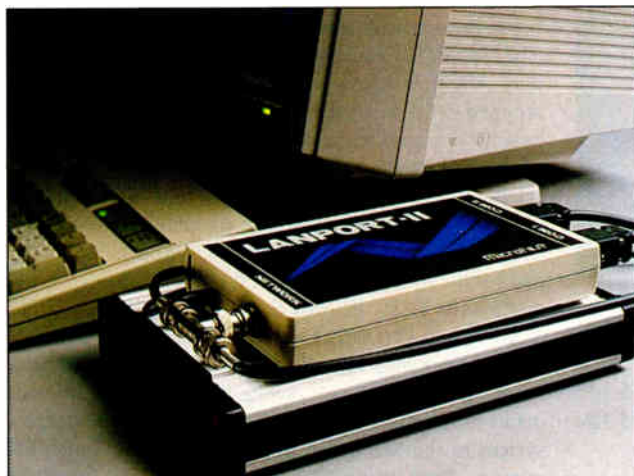
LANPORT-II lets you dial into your LAN without the need for a PC communications server.
