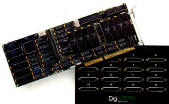
DigiCHANNEL PC/Xi. 8 or 16 asynchronous channels. 12.5 or 16 MHz 80186 processor. 128K or 512K RAM. Synchronous channel option. For multichannel applications that demand speed, configuration flexibility and programmability.
