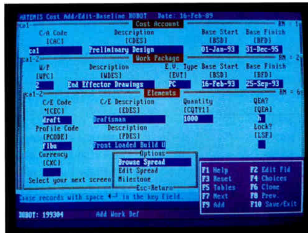
The screen layouts of Artemis Cost complement the underlying data structures, so that Cost Account, Work Package, and Elements maintain a hierarchical structure.
