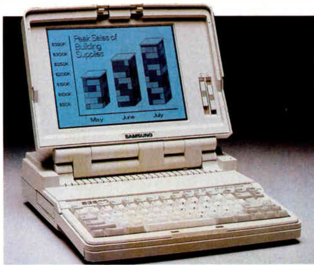
The Samsung S3600 is a 12-MHz laptop with a 40-MB hard disk drive and a VGA-compatible screen.
