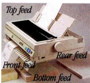
Only one paper path is available at any given time for continuous paper.
