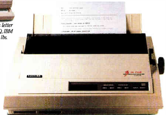
P32ISL/SLC (color): 216/72 cps, 24-pin letter quality, up to 360x360 DPI graphics, Toshiba/Qume and IBM emulations standard, Epson and Diablo emulations optional, 32KB print buffer, front panel controls, advanced paper handling.
