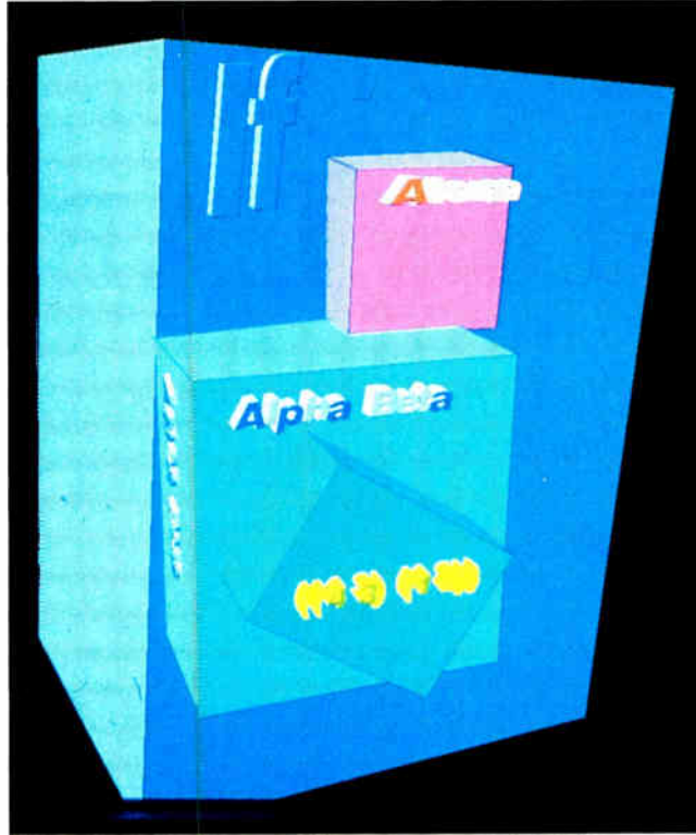
Photo 2: With hardware rendering of three-dimensional shapes now practical, Media Lab researchers are conducting experiments with 3-D representation of programs. In this 3-D graphical debugger, the boxes represent program elements; they change size, position, and color as the program runs. (Photography: Lieberman, Visible Language Workshop)
