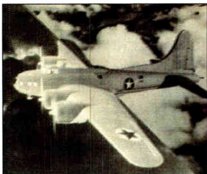
Photo 1: Conditional point processing converts the image below the diagonal to a negative.
