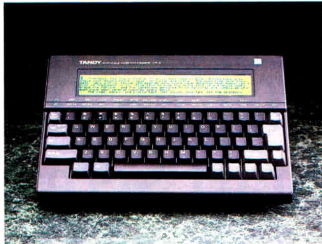
Tandy's WP-2 is a dedicated word processor with a built-in 200,000-word thesaurus and communications software.
