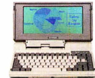
T1200HB: 10.8 lbs, 9.54MHz 80C86, 20MB hard disk, 1MB RAM, includes 384KB LIM-EMS. Removable/rechargeable battery pack.
