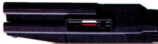
T5100: 16MHz 80386 microprocessor, 40 or 100MB hard disk, 2MB RAM expandable to 4MB, 14.6 lbs. Built-in EGA display with high resolution gas plasma screen.
