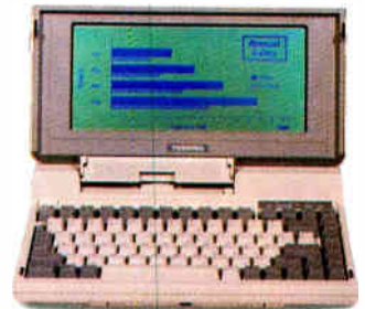
T1200FB: 9.8 pounds, 9.54MHz 80C86, 1MB RAM, 2 720KB 3½" floppy drives, removable/rechargeable battery pack.
