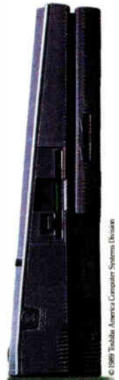
T3200: 12MHz 286, 2 IBM compatible slots, 40MB hard disk, 1.44MB floppy, 1MB RAM expands to 4MB, EGA screen.
