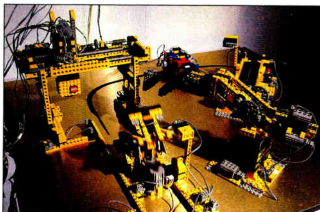
Photo 6: A model of a factory assembly line, constructed from "intelligent" Lego elements controlled by an Apple-based Logo program.
