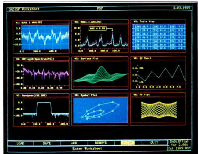
DADiSP 2.0, displaying raw data and several functions. Note that in the top middle window, a change in the raw data would change the maximum value in the annotation.
