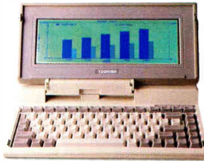
T1000: 6.4 lbs, 4.77MHz 80C88, 512KB RAM expandable to 1.2MB, MS-DOS in ROM, 720KB 3½" diskette drive. Built-in RGB, parallel, serial and external drive ports.
