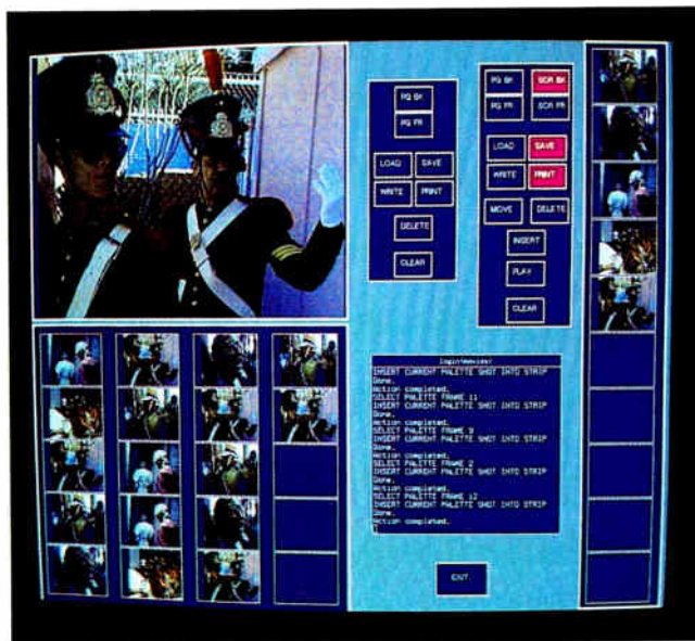
Photo 4: This video storyboarder runs real-time digital video on a Unix-based workstation running X Window. (Photography: Pepe/Sheldon, Film/Video Group)
