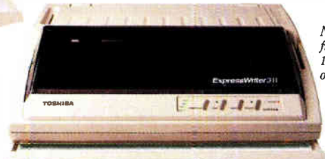
ExpressWriter 311: 24-pin dot matrix, 180 cps draft/60 cps letter quality, 3 resident emulations (Toshiba/Qume, Epson LQ, IBM Proprinter), 16K buffer, 5 resident fonts plus card slots, 11 lbs.
