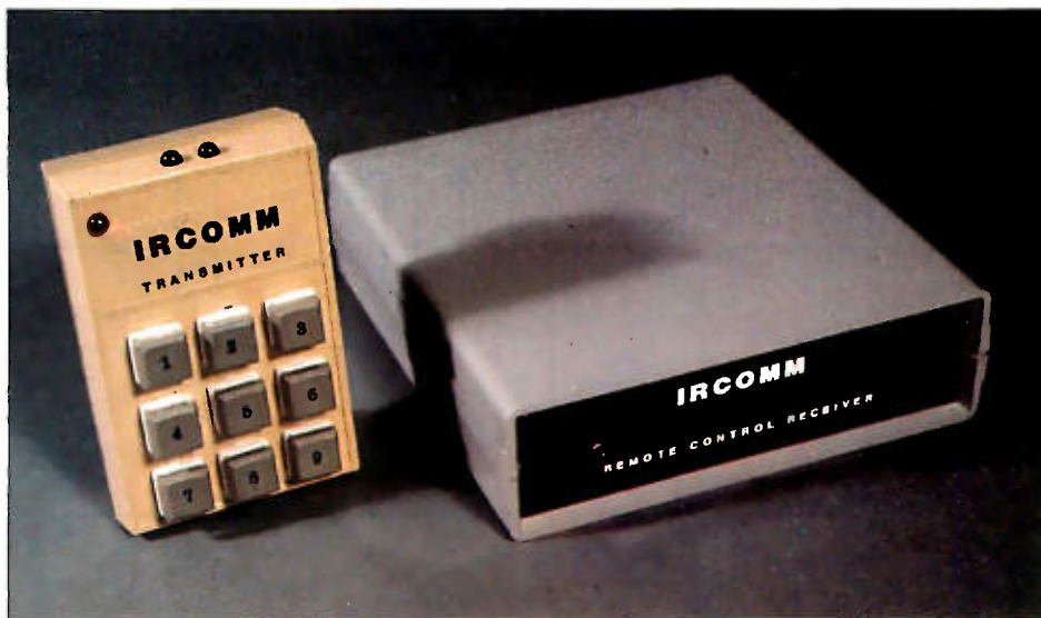
Photo 1: Enclosed IRCOMM transmitter and receiver units.
