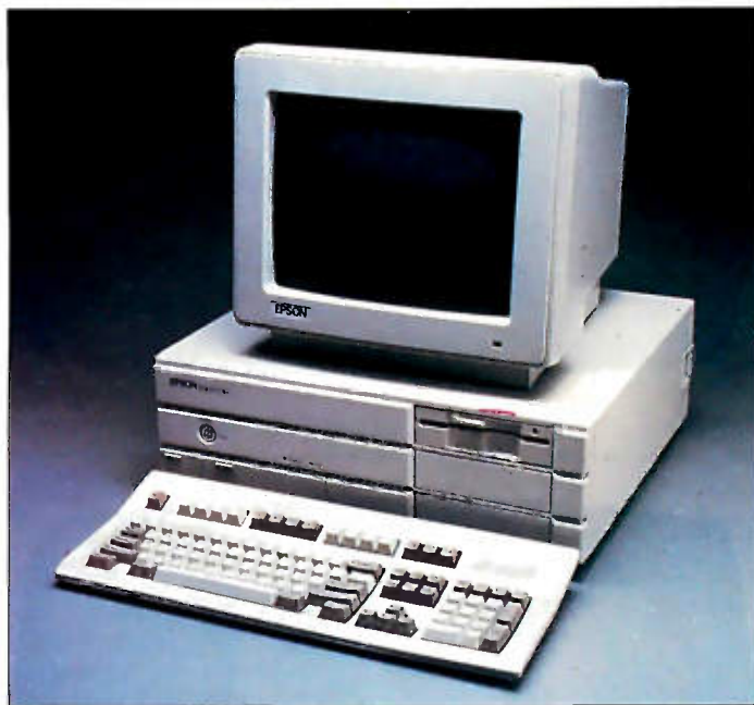
Epson's Equity III+ has an 80286 that can run at three speeds.
