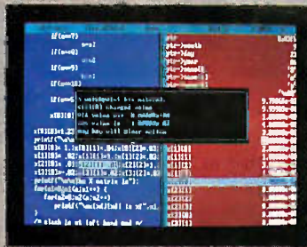
Source and variables windows shown side by side. Pop up message indicates that a watch point condition has been satisfied.
