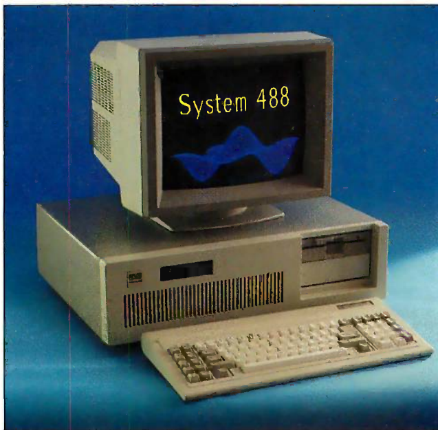
The System 488 comes with an IEEE-488 interface and specialized software.
