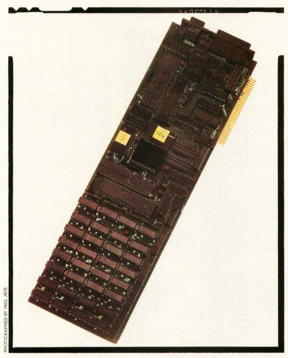
Photo 1: The DSI-32 coprocessor board.
