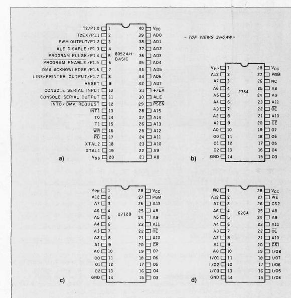
Figure 5: Pinouts for (a) the 8052AH-BASIC chip, (b) the 2764 8K-byte EPROM, (c) the 27128 16K-byte EPROM, and (d) the 6264 8K-byte RAM.
