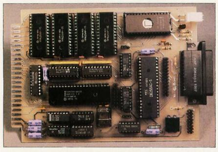
Photo 1: The Circuit Cellar BASIC-52 computer/controller prototype.
