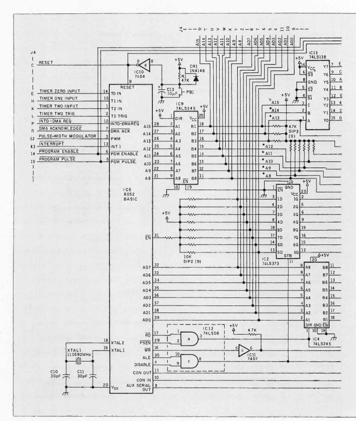
Figure 3: Schematic diagram of the BCC-52 board.
