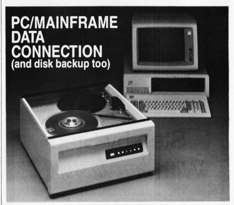
With the Digi-Data 2000 PC ½" tape system you can move data between your IBM PC, XT, or AT and a mainframe or minicomputer. IBM/ANSI compatible 9-track 1600 bpi ½" tape is the only truly standardized and interchangeable medium between the PC and mainframes or minis.
