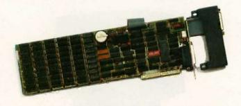
Simply, the best deal on a PC multifunction board-bar none. Basic Time's six function board, the BT6Plus, includes memory sockets for adding 64K to 384K, parallel printer port, asynchronous (RS-232C) serial communications port, battery-powered clock/calendar and electronic disk emulation & print spooling software. Optional game port. Comes complete with an easy-to-understand installation instructions/user's manual.
