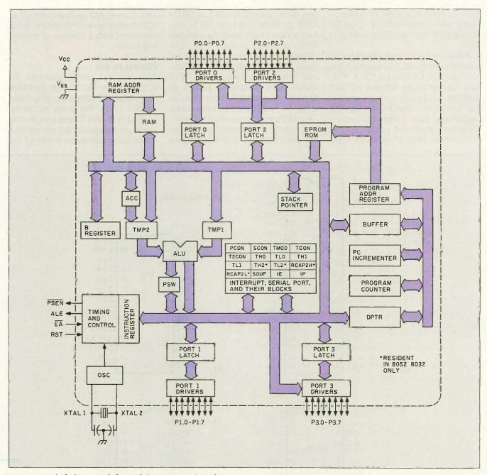
Figure 4: Block diagram of the Intel 8052AH-BASIC chip.
