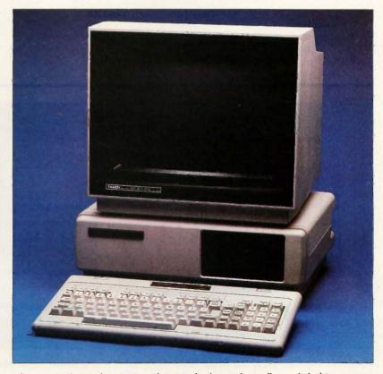
Photo 1: The Tandy 1000 with RGB display and two floppy-disk drives.
