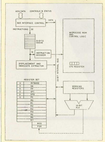
Figure A: A block diagram of the 32032 CPU.
