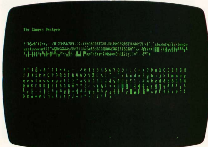
Photo 3: A display of the high-resolution, monochrome-text-mode character set on the Compaq Deskpro.
