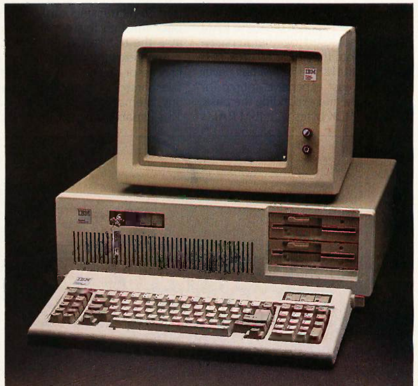
Photo 1: The IBM PC AT with a 20-megabyte hard-disk drive, 1.2-megabyte floppy-disk drive, and 360K-byte floppy-disk drive.
