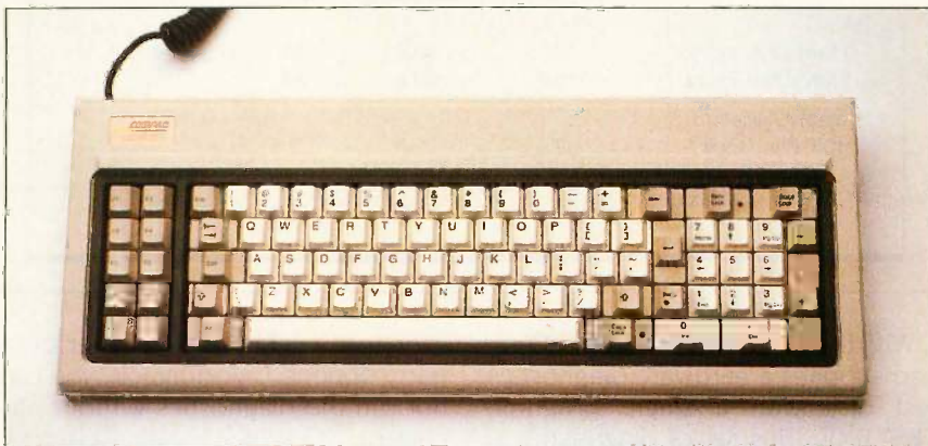
Photo 4: The Compaq Deskpro keyboard. Note the LED indicators on the Caps Lock and Num Lock keys.
