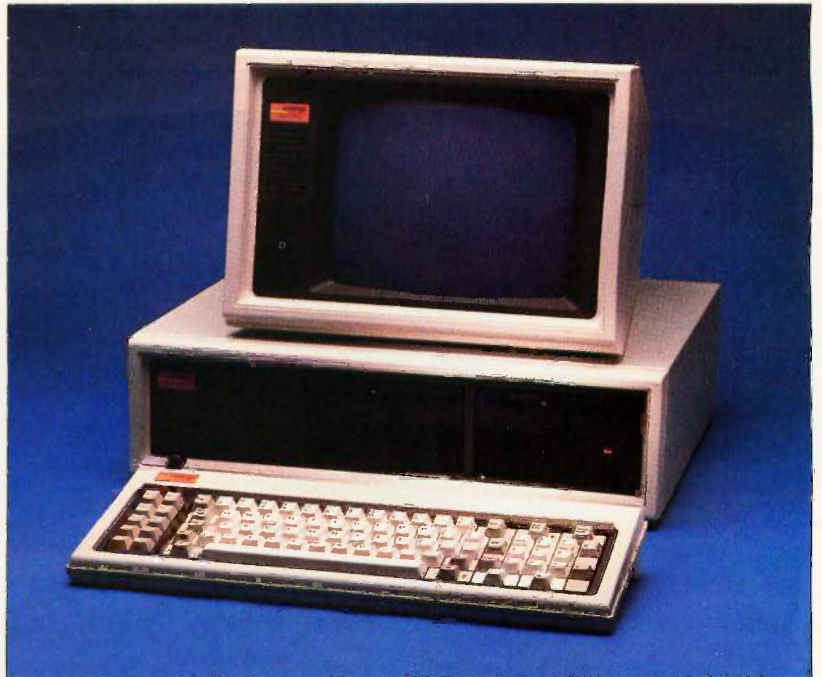
Photo 1: The Compaq Deskpro Model 4 with 10-megabyte hard-disk drive, 10-megabyte tape-cartridge system, optional second floppy-disk drive, and optional 12-inch green monitor. Note the clock-speed indicator light and keyboard plug to the left of the disk drives.
