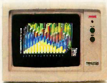
HX-12. High resolution RGB monitor -690 x 240 lines noninterlaced - .31 mm dot pitch tube-Nonglare screen - $695
