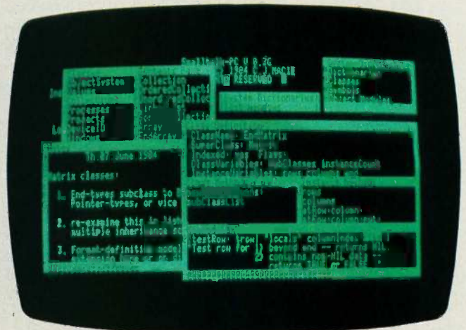
Photo 2: A sampling of Smalltalk-PC windows. There is a scanner in the upper left showing class categories (left pane) and their classes (right pane). There is a form of class editor in the lower right. In the lower left is a text window, and in the upper right is a list, out of which the scanner was called. The two-line inverse window in top center is the pop-up menu of the screen (mouse button 2 is being held).
