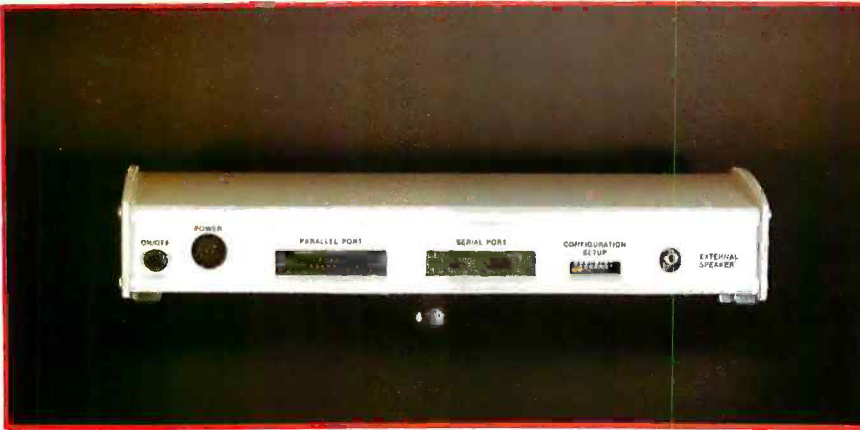
Photo 4: The rear panel of the Votrax contains the on/off switch, a parallel and a serial port, DIP switches, and an external speaker jack.
