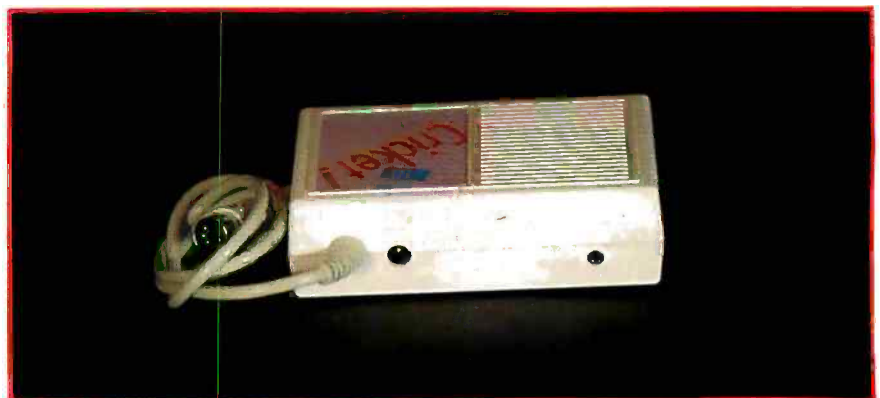
Photo 1: The Cricket's rear panel has a five-pin DIN I/O cable and room for an external speaker.
