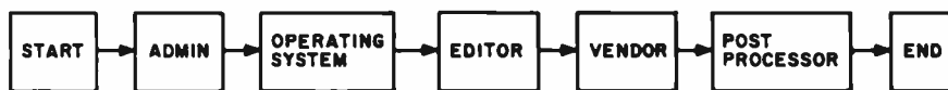
Figure 3: Layers of software between the user and graphical output. Lack of knowledge of software layers denies most users access to graphics.
