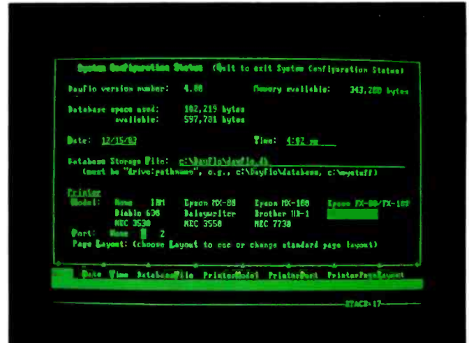
Photo 8: The System Configuration Status screen allows changes to major system features. Dayflo can be used with more than one database—to switch to a different database, simply overwrite the Database Storage File name with the new information.
