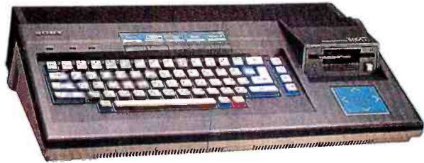
Photo 7: The Sony SMC-777 Z80-based home-graphics computer includes a single 3 1/2-inch drive and lists for about $650 in Japan.
