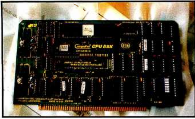
Photo 5: The System 68K's central processing unit's 68K-byte board.
