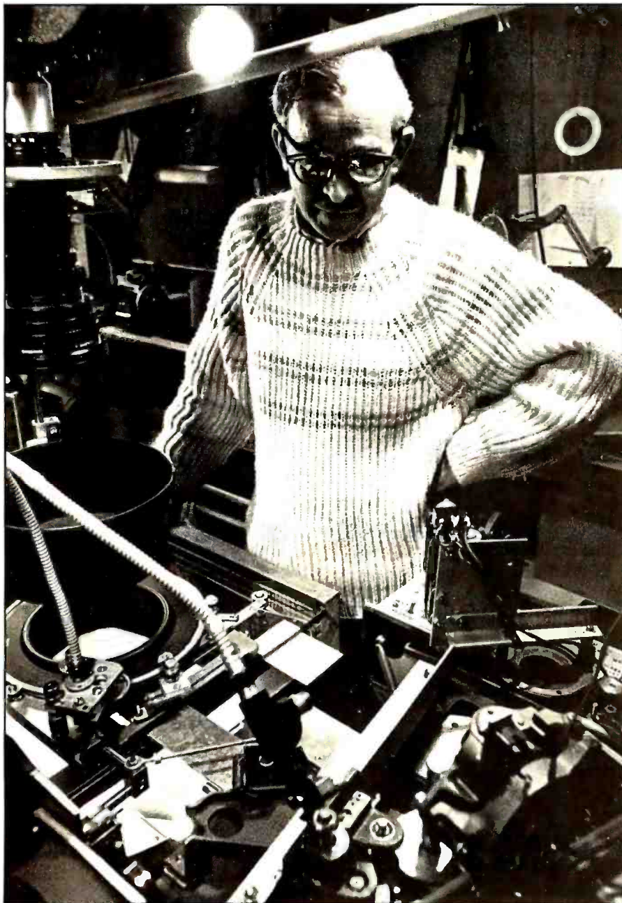
Photo 9: Pioneer computer animator John Whitney Sr. in 1959, operating one of the first computer-graphics engines, a mechanical analog computer built largely from surplus World War II anti-aircraft guidance hardware. The camera is in the upper left, aiming down through the apparatus that "paints" the film with light. (Photo by Charles Eames.)
