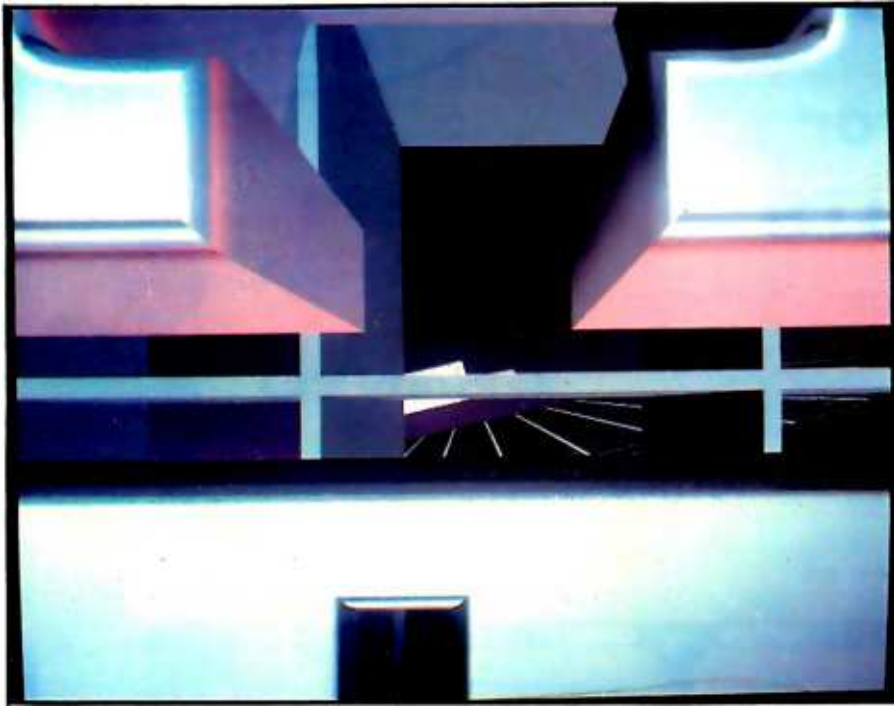
Photo 10: The opening title animation for the television show "Entertainment Tonight," done by Carl Rosendahl of Pacific Data Images. The sequence is created using smooth-shaded polygons and anti-aliasing.
