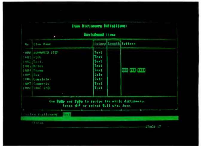
Photo 10: The Item Dictionary lists all field names that Dayflo "knows" and their attributes. If you enter data that does not conform to the dictionary specifications, the program will request verification before accepting the information. Nonindexed items can be retrieved only as part of entire records; indexed items can be retrieved independently.
