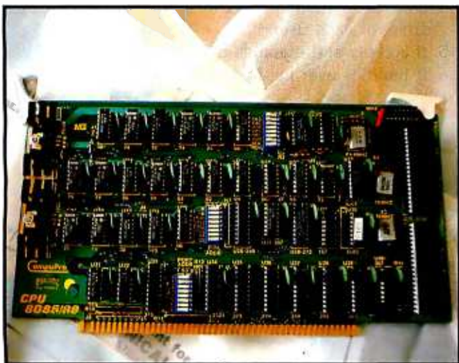
Photo 3: The 8085/8088 central processing unit of the System 816/C.
