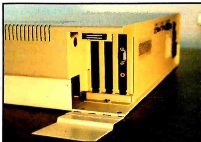
Photo 2: The expansion-card connector cavity. The keyboard connector is to the left of the card connectors. The dark rectangle at the top is the magnetic catch. To get at the expansion slots, you can remove the piece of metal to which the cavity door is hinged.
