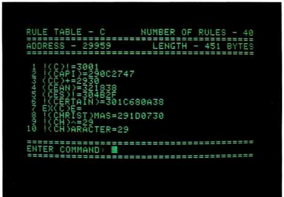
Photo 2: The rule editor for the text-to-speech software displays the phoneme-translation rules for each letter in groups of 10.
