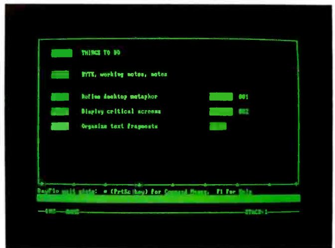
Photo 4: A database-style form under construction. The INS and NAME flags appearing on the status line at the lower left of the screen indicate that you're in insert mode and that a field name is being entered. Once this record has been completed, it can be retrieved by searching for the contents of any single field name (or group of names).
