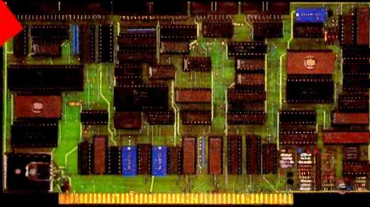
A hard disk and cartridge tape controller together on one board? Magic? Not really. It's Teletek's HD/CTC. The hard disk and cartridge tape drive controller provide the support necessary to interface both rigid-disk drives and a cartridge tape deck to the S-100 bus.
