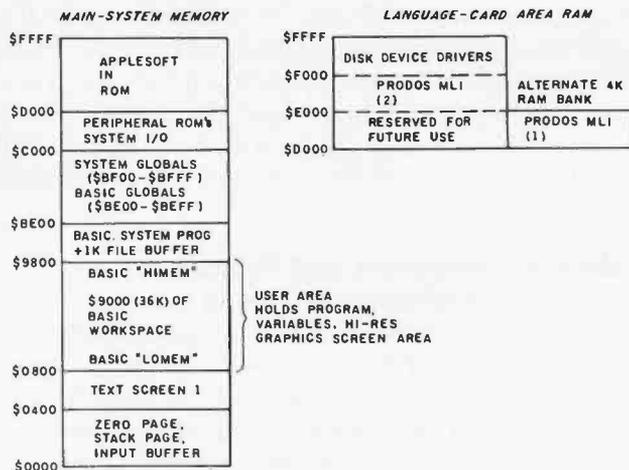
**Figure 3:** A memory map of a 64K-byte Apple II or IIe with ProDOS and SYSTEM.BASIC installed. ProDOS is stored primarily in the language-card area of memory, and BASIC.SYSTEM resides in the area formerly occupied by DOS 3.3. Coincidentally, a ProDOS system provides about the same amount of free BASIC user space as a DOS 3.3 system.
