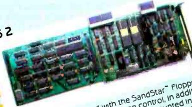
This System is equipped with the SandStar™ Floppy Drive Controller Card. The Card can control, in addition to the Hard Disc Drive, two floppy drives mounted inside your PC and optionally two additional 5¼" or 8" drives mounted externally. This leaves three system slots for other expansion boards.
