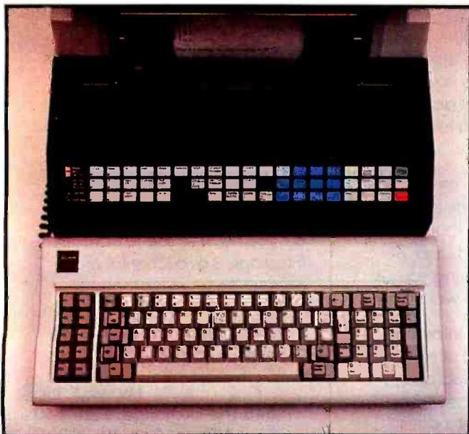
**Photo 3:** The CS-9000 keyboards. At the top, on the front of the main processor box, are the 57 programmable, pressure-sensitive keys.
