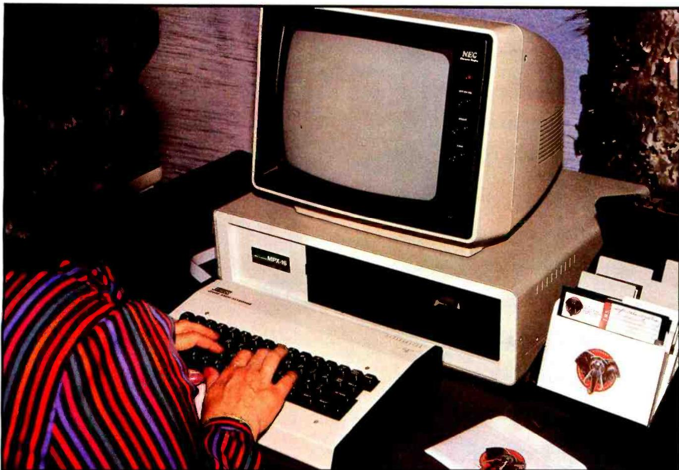
**Photo 5:** The Term-Mite ST circuitry described in these articles is used with a separate keyboard and video monitor to form a complete functional terminal. Here a Jameco JE610 keyboard works with the Term-Mite, a NEC (Nippon Electric Company) green-phosphor monitor, and the Circuit Cellar MPX-16 computer.
