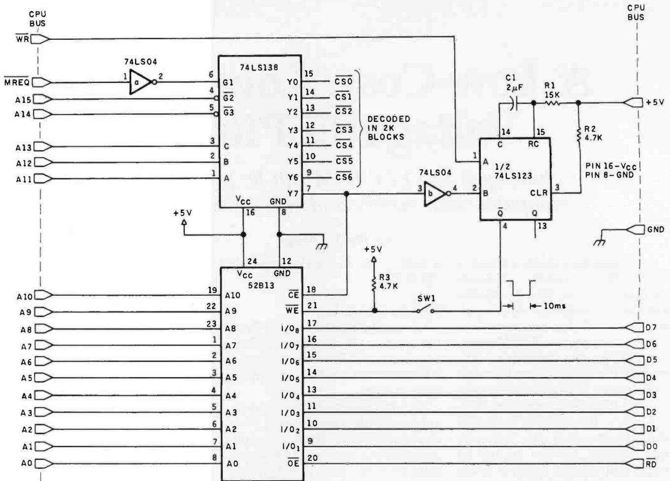
**Figure 1:** A schematic of the 52B13 EEPROM circuit. The EEPROM is decoded the same as the other 2K by 8-bit memory blocks. A one-shot provides the 10-ms write-enable pulse needed for the EEPROM to be programmed.
