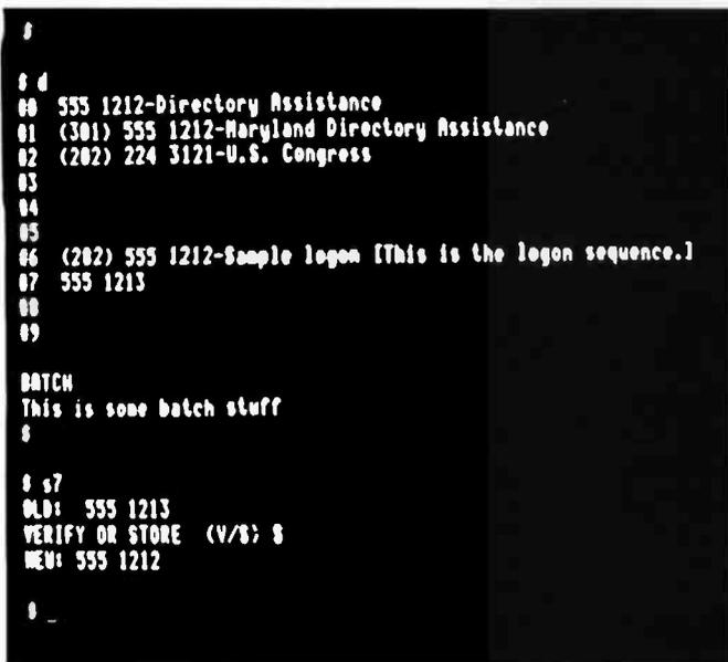
Photo 3: The R212A's directory display. The notations next to the phone numbers are stored as ASCII text by the modem. "BATCH" is a way to run a set of commands. The bottom of this display contains an example of storing a new phone number.
