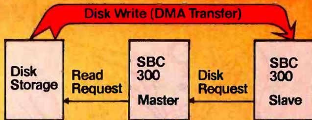
The SBC 300 offers you 64K bytes of dual ported parity RAM. Dual porting allows DMA transfers from disk storage *directly* to an individual slave processor. This maximizes multi-processor system performance.
