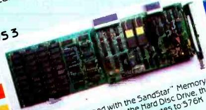
This System is equipped with the SandStar™ Memory Card. In addition to controlling the Hard Disc Drive, the Memory Card allows you to add 64K bytes to 576K bytes of memory using only one card slot.
