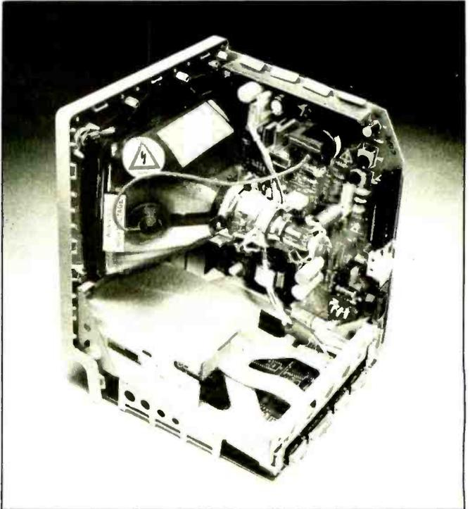
**Photo 3:** Inside the Macintosh computer. From the front (photo 3a), you can see the video display and the 3½-inch disk drive. From the rear (photo 3b), you can see the two main circuit boards (right and bottom), the rear of the video-display tube, the 3½-inch disk drive, and a row of connectors at the bottom of the unit. The connections go, from left to right, to the mouse, a second disk drive, two peripherals (these are two serial ports), and an external amplifier (for sound output).
