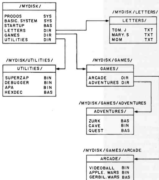
**Figure 1:** A typical ProDOS directory structure. The pathname, shown above each directory listing, describes the path followed to reach a particular directory from the volume name on down. If the volume specified is mounted anywhere in the system, ProDOS will find it regardless of which drive it's in.
