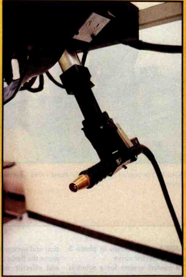
Photo 11: The end effector on a robot does not necessarily have to be a grasping tool, as illustrated here by this arc-welding tool.
