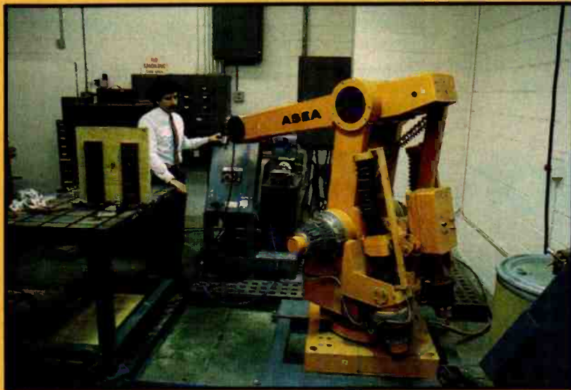
Photo 3: The ASEA robot model number IRb-60 shown here at the ASEA application laboratory in White Plains, New York, illustrates the revolute-arm geometry.
