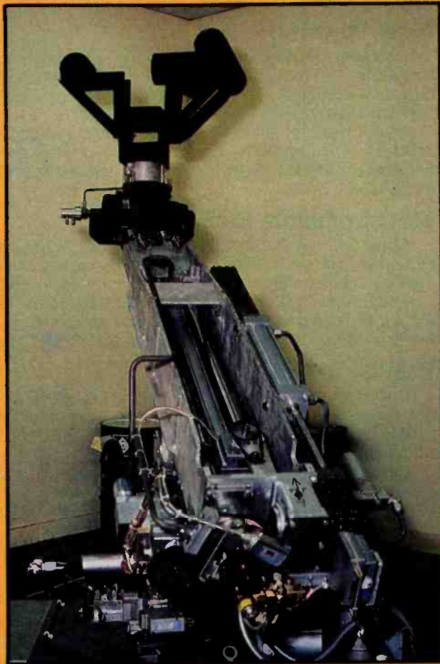
Photo 6: All Unimation robots are thoroughly tested before they are shipped to a customer. This robot is executing a sequence of steps with a 450-pound weight attached in order to test all motions.
