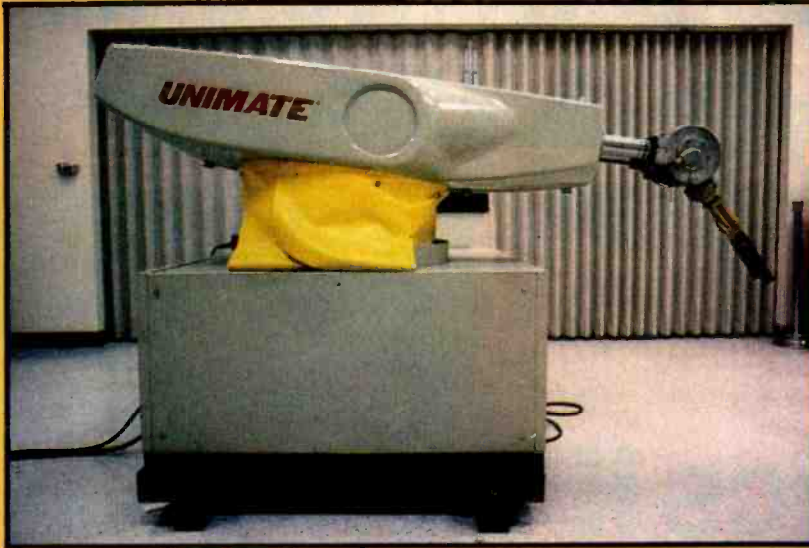
Photo 2: The Unimate 2000 is a good example of a robot with polar-coordinate arm geometry.
