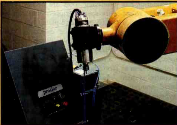
Photo 12: A high-speed cutting tool, used to cut plastic and fiberglass sheets into different shapes, is shown attached to the end of an ASEA robot.
