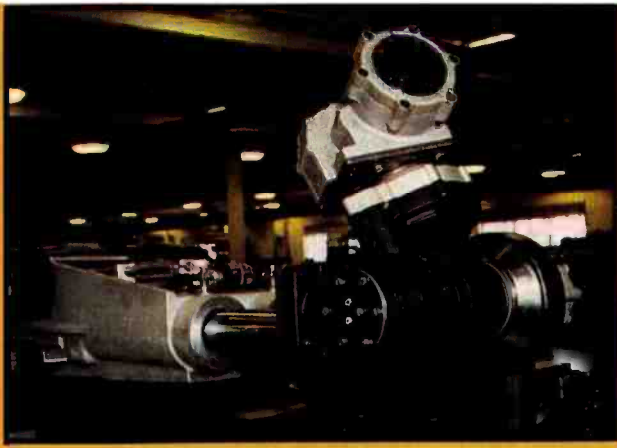
Photo 4: Three wrist articulations are usually required to position an end effector. Bend, swivel, and yaw motions are possible with the configuration shown here.
