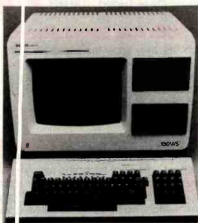
Mo torola 68000, 256K memory, 10MB Winchester disk, 760KB floppy, terminal, system software, choice of Pascal, FORTRAN, C, Assembler, BASIC, COBOL
