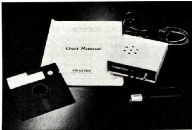
Photo 1: The Cognivox VIO-1003 Voice Recognition and Voice Output System.
