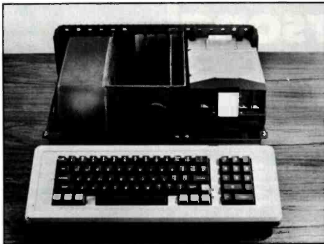
Photo 3: The Apple III with its main cover removed. The power supply is housed in the enclosure visible to the left, I/O card slots are in the center, and the disk drive is on the right. The entire Apple III is built around a single thin-wall aluminum casting that provides both support and shielding.
