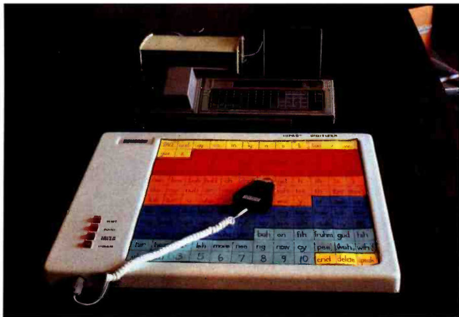
Photo 5: A Houston Instrument Digitizing Tablet is added to the HHC and Type-'N-Talk to allow for an expanded and flexible keyboard.
