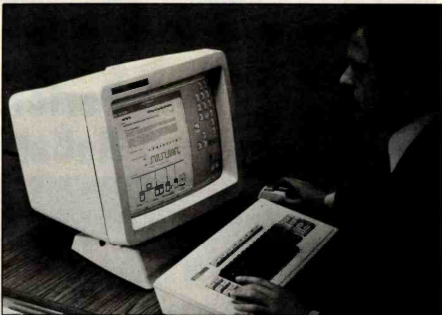
Photo 1: A Star work station showing the processor, display, keyboard, and mouse.
