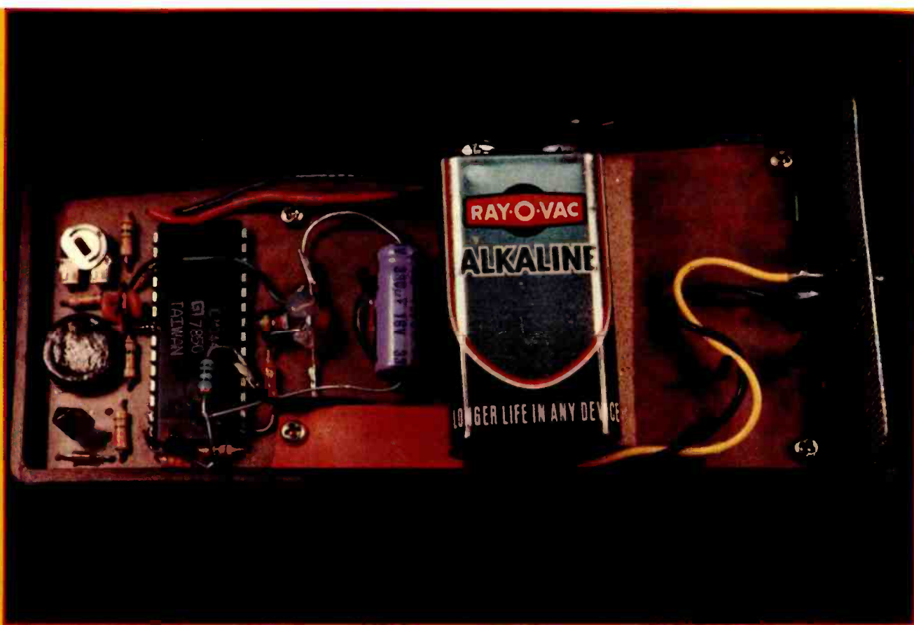
Photo 6: Interior view of the modified BSR X-10 hand-held transmitter, modified according to figure 7.
