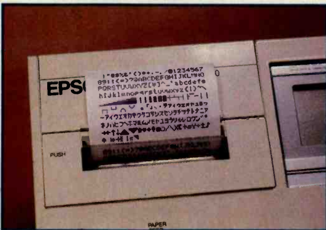
Photo 2: The HX-20 printer and a printout of its character set. The Japanese katakana characters will be replaced in the U.S. version of the unit by geometric symbols that can be combined to make larger graphic images.
