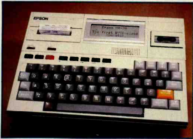
Photo 1: A prototype of the HX-20 microcomputer. The final unit will have a different keyboard layout.
