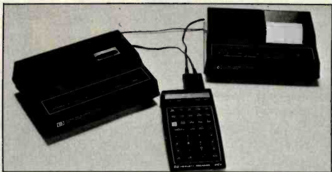
Photo 2: HP-41C connected to an HPIL Module, Digital Cassette Drive, and Thermal Printer/Plotter in the loop.
