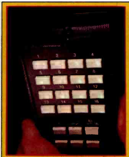
Photo 5: The familiar BSR X-10 hand-held control unit. This was built to work using ultrasonic pulses, but it can be modified to use infrared light. The added infrared LED can be seen on top of the housing.
