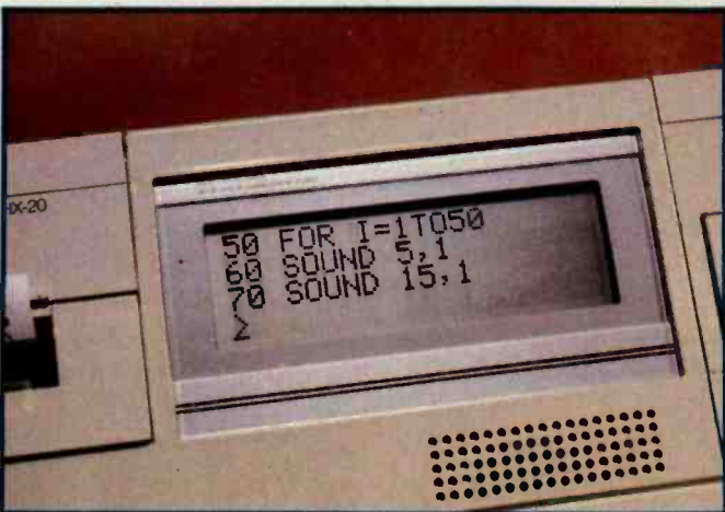
Photo 3: The liquid-crystal display of the HX-20, which gives four rows of 20 characters each.
