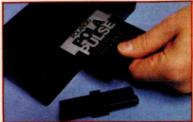
Photo 2: The Telecomputer is powered by a built-in Polaroid Polapulse flat battery.
