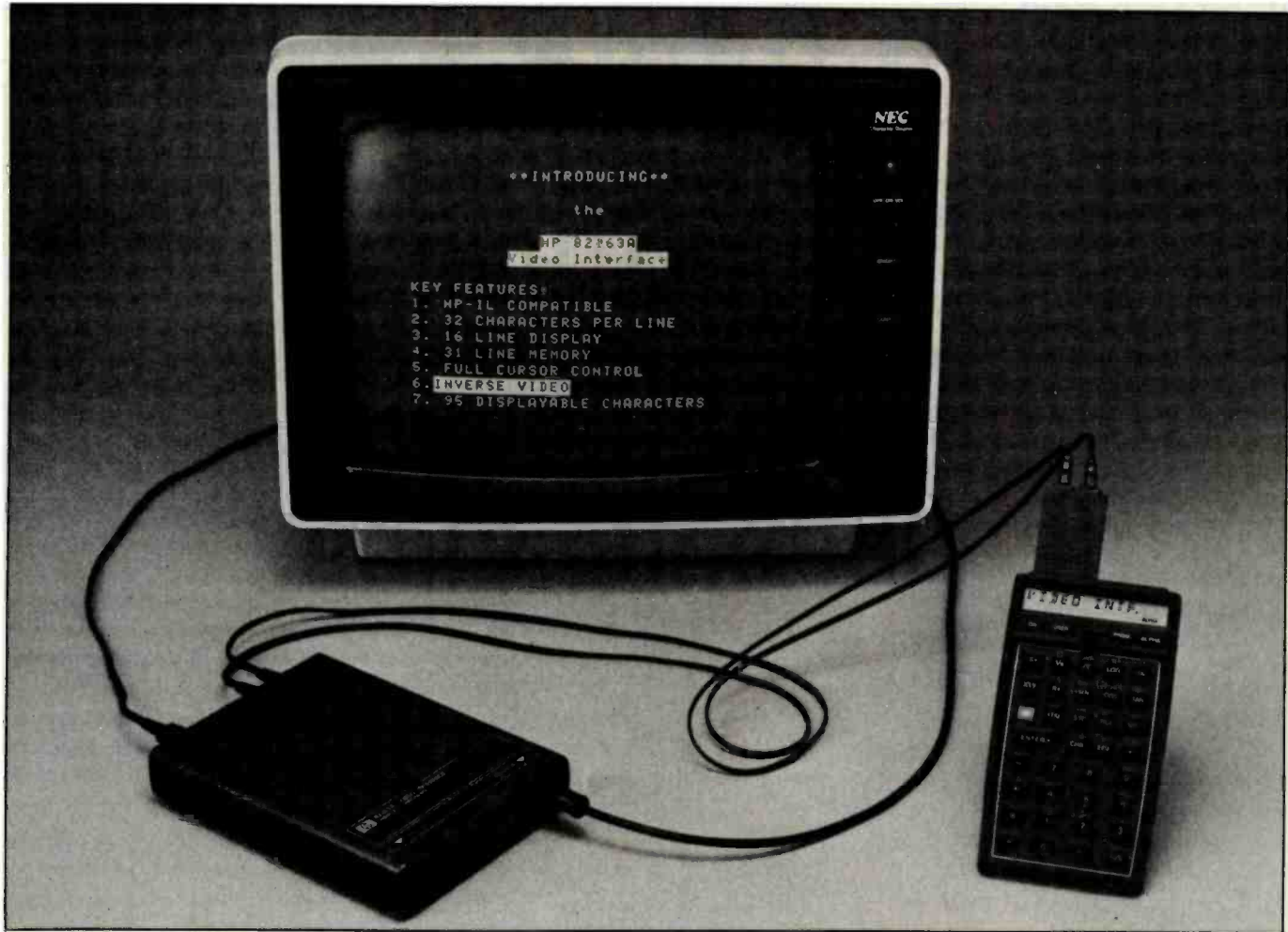
Photo 5: Hewlett-Packard's HP82163A Video Interface connects a monitor or TV to HP's interface loop. This permits handheld computers like the HP-41C—previously limited by a single-line display—to display information in a 16-line by 32-character video format. Aided by the new interface (available by the end of 1982), HP-41C owners can review up to 16 program steps at a time.
