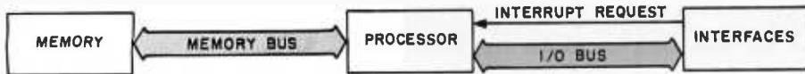
Figure 4: A computer system with memory bus, I/O bus, and added interrupt line. Interrupts allow the processor to start I/O processes, then go on to other tasks. The peripheral uses the interrupt line to indicate readiness for another transaction.
