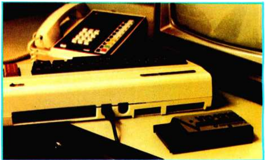
Photo 1: This low-cost modem for Commodore's VIC-20 home computer takes a modular plug from a telephone handset and plugs directly into VIC-20's telecomputing slot. The modem shown here is a prototype with a provisional model number.
