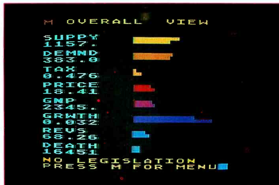
Photo 1: A bar chart made using character graphics. Even though each character is eight pixels wide, the horizontal bars can be any number of pixels wide by using redefined characters representing bars of varying width.
