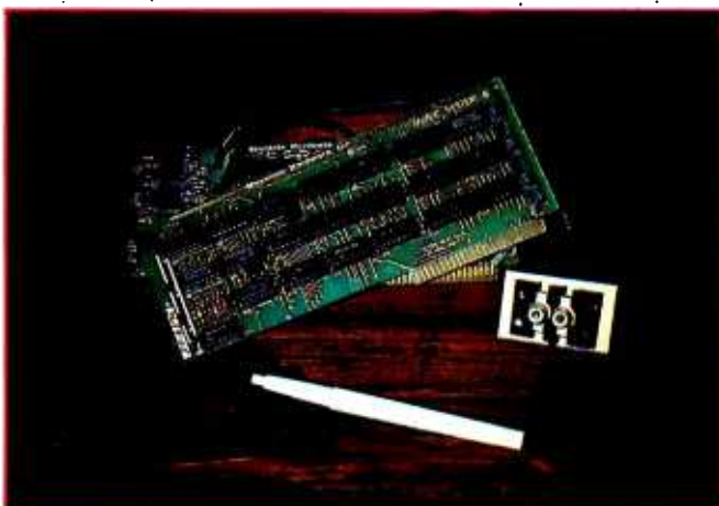
Photo 1: The MusicSystem circuit boards with light pen and stereo outputs. The boards may occupy any two adjacent expansion slots, except slot 0, in the Apple II.
