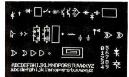
Photo 2: Component types available for drafting. All figures shown are created by the program in listing 2.
