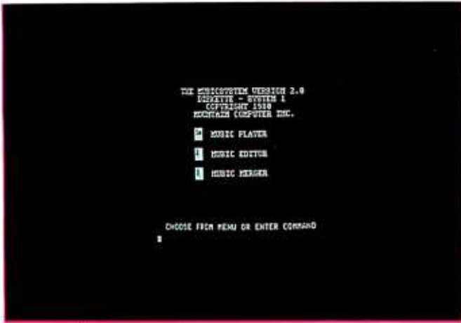
Photo 2: The System 1 main menu. Selections can be made by touching the light pen to the block at the left of each item. The tiny square in the top block indicates the presence of the game-paddle cursor. If the button on paddle 0 is pressed, the Music Player is selected.
