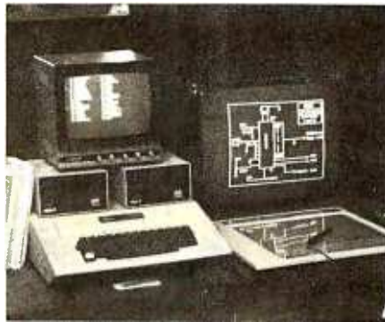
Photo 1: The author's computer-aided drafting system for the Apple II computer. Addition of a Graphics Tablet, a Sup'rterminal 80-column display board, and some software can take the drudgery out of designing electronic circuits.
