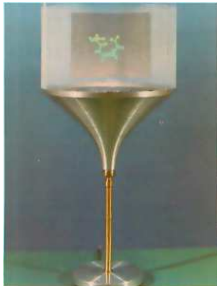
Photo 9: Integral hologram of a molecule created by photographing 1080 computer-generated images on 35mm film and then transferring them to a hologram. In the future computers will be able to generate holograms directly. Photo courtesy of Donald L. Vickers, Lawrence Livermore National Laboratory.
