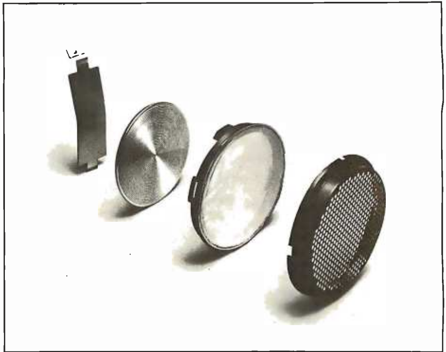
Photo 5: Expanded view of the Polaroid ultrasonic sonar transducer. Behind a honeycomb grill, a 0.003-inch (0.07 mm)-thick gold-coated foil stretches over a concentrically grooved aluminum plate. The retainer at left holds the parts in place.
