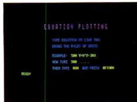
Photo 1: Variation of text height and color. Both text height and color can be changed under program control.
