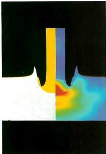
Photo 8: A problem in hydrodynamics illustrated through the use of computer graphics. The photo is part of a series illustrating a steel rod impacting a steel plate. Color changes represent areas of varying stress. In the future, such graphics will be widely used in education. Photo courtesy of Lawrence Livermore National Laboratory.
