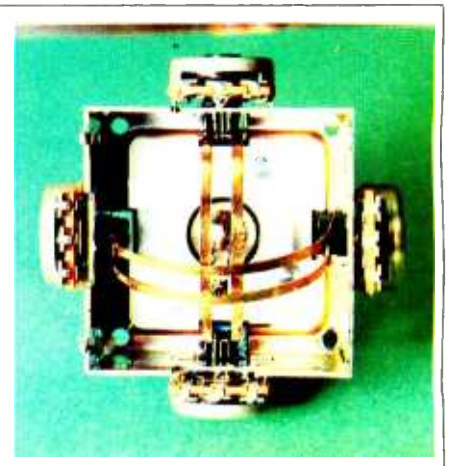
Photo 2: Note how moving the stick moves the gimbal arrangement, which in turn changes the settings of the potentiometers.
