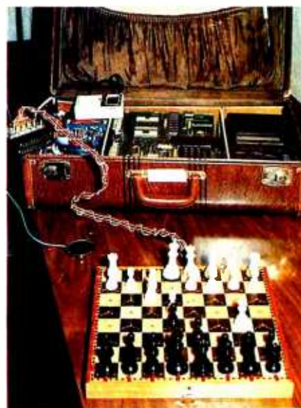
Photo 3: The complete chessplaying system. The completed electronic chessboard stands in the foreground. The chessboard and the sound-effect speaker are connected to the KIM-1 computer residing in the suitcase in the background.
