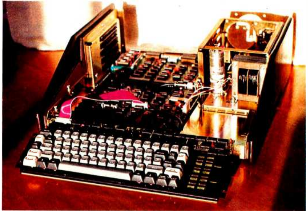
Photo 1: Processor Technology SOL, with cabinet cover removed to reveal its inner secrets.
